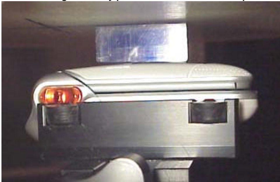
Position of device against body phantom with ICE26 in back position.
