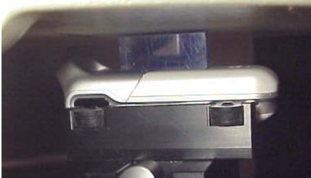
Position of device against body phantom with 15mm in back position.
