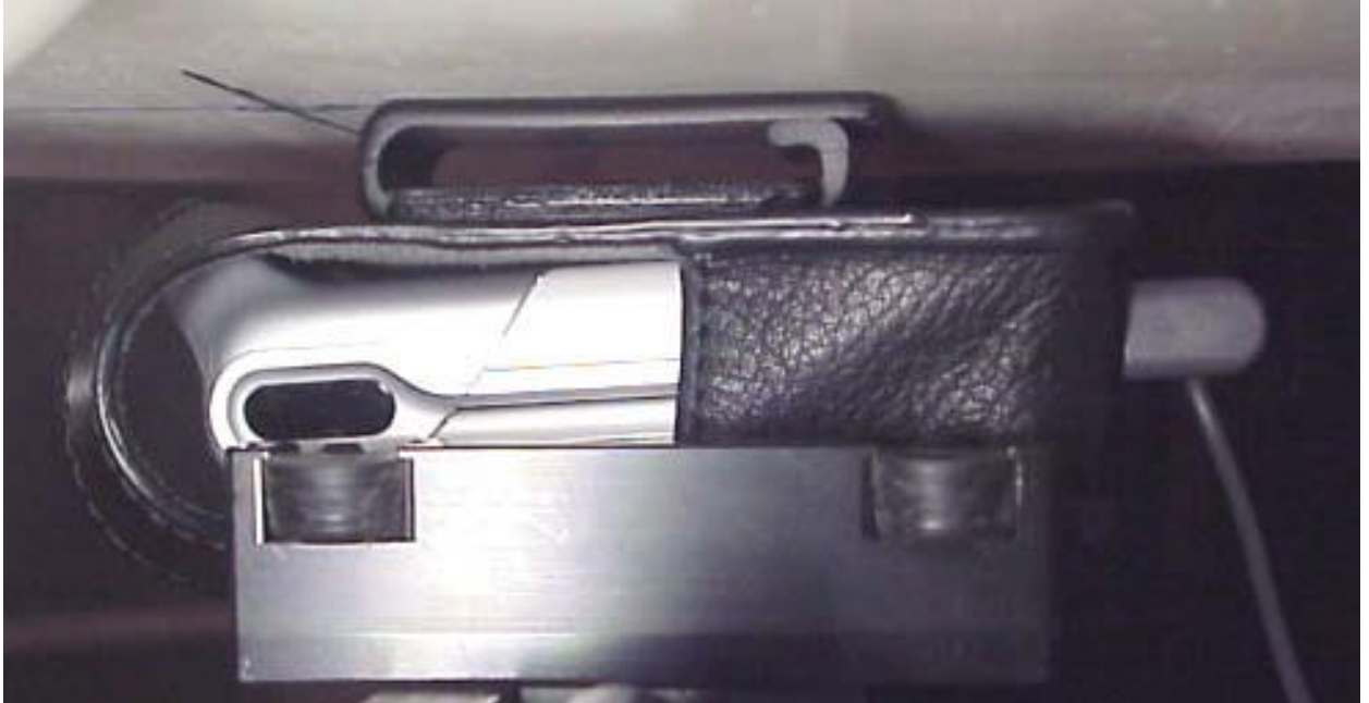
Position of device against body phantom with ICE26 in back position.
