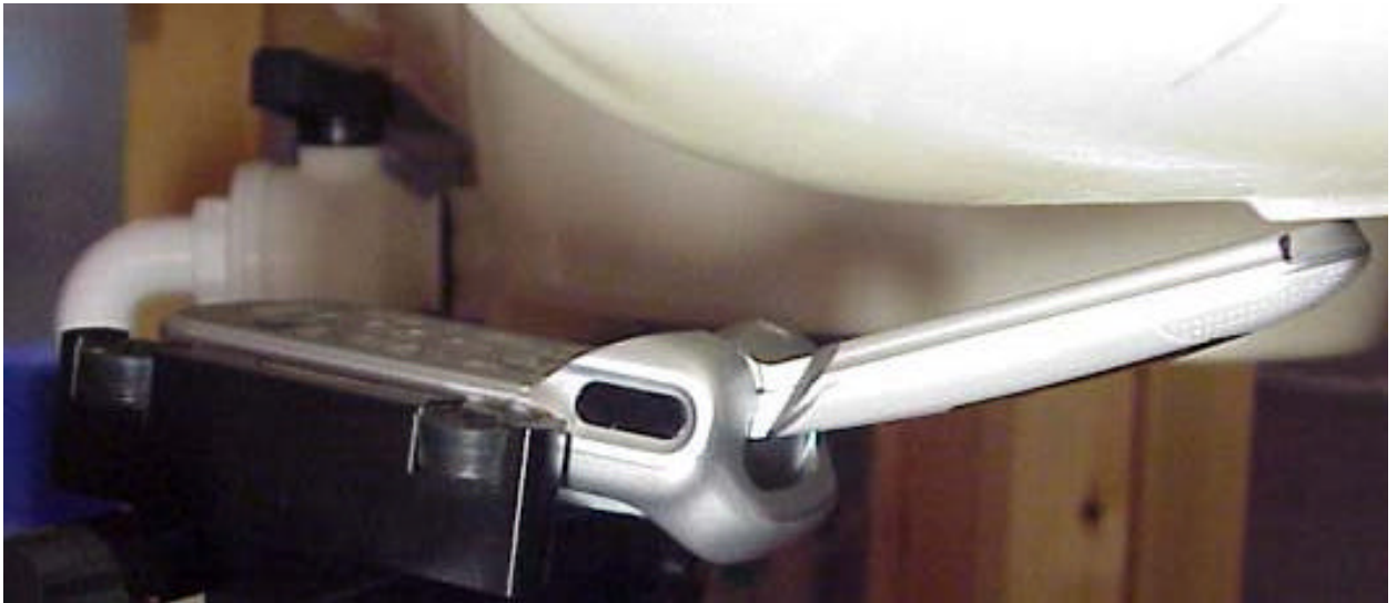
Position of device against head phantom using the “tilt” position
