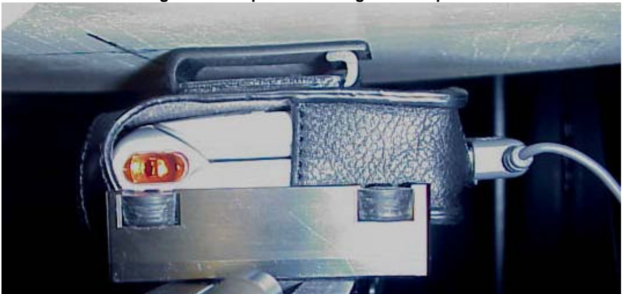
Position of device against head phantom using the “tilt” position
