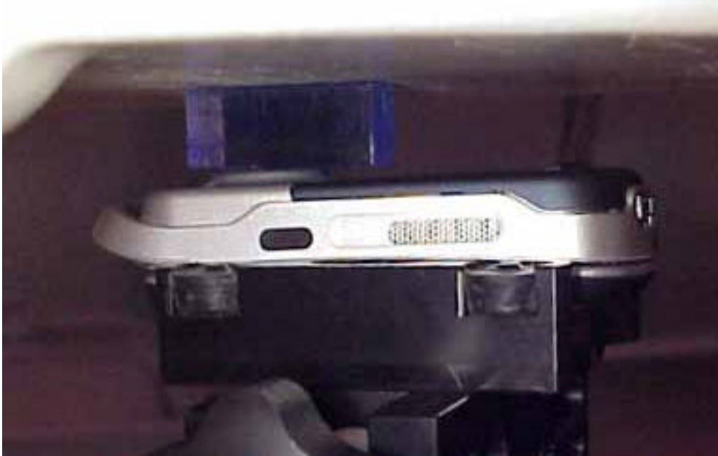
Position with back of device against flat phantom using a 15MM spacer.
