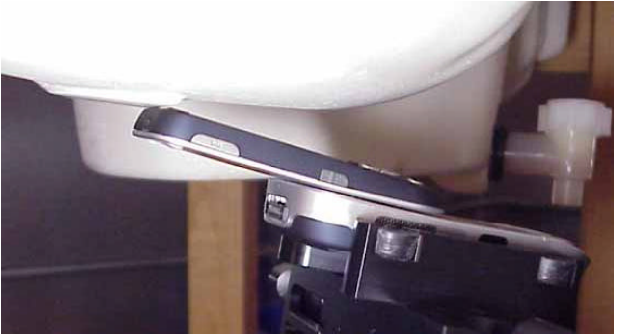
Position of device against head phantom using the “tilt” open position
