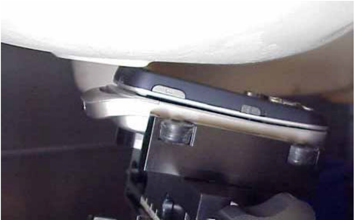
Position of device against head phantom using the “tilt” closed position
