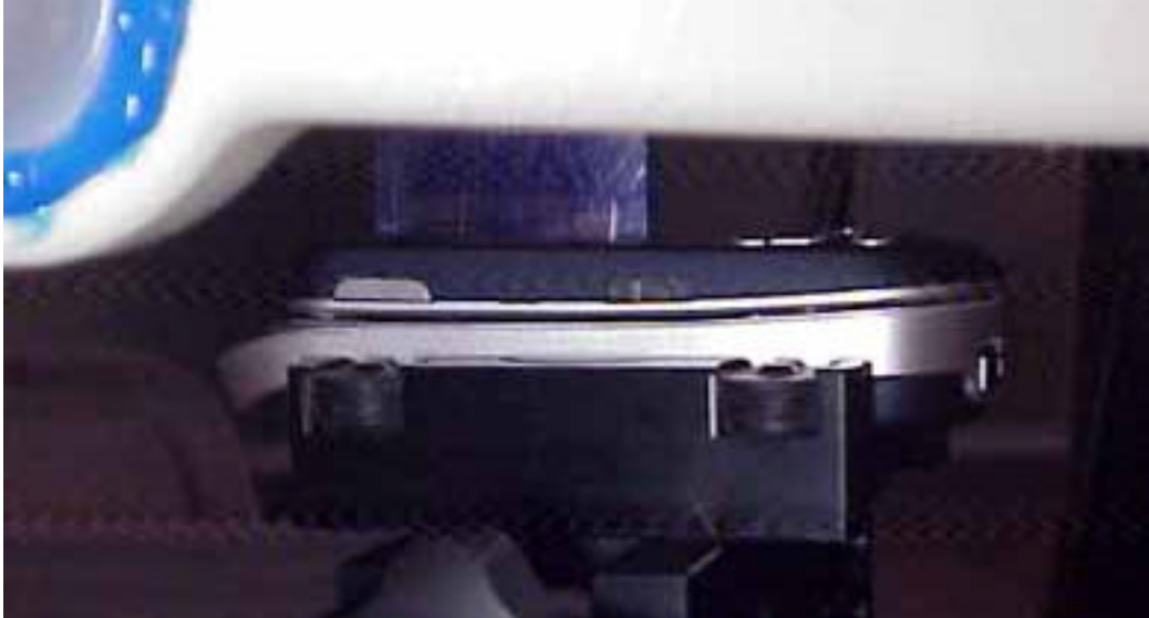
Position with front of device against flat phantom using a 15MM SPACER.
