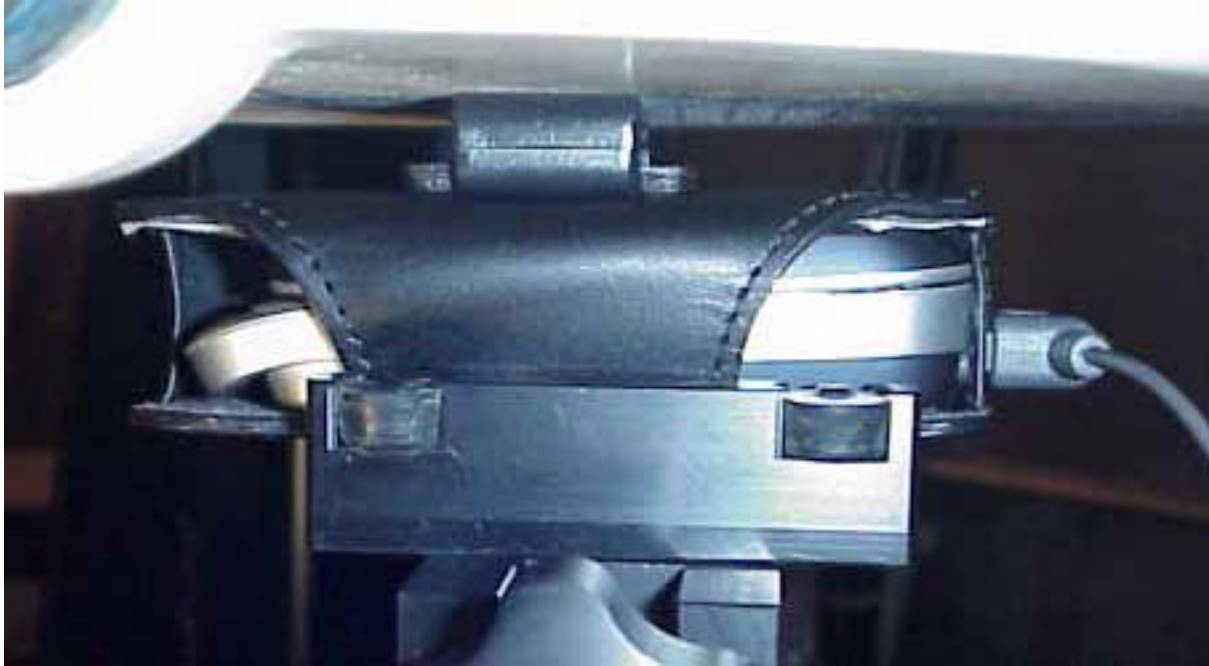
Position with front of device against flat phantom using a ICE30 carry case.
