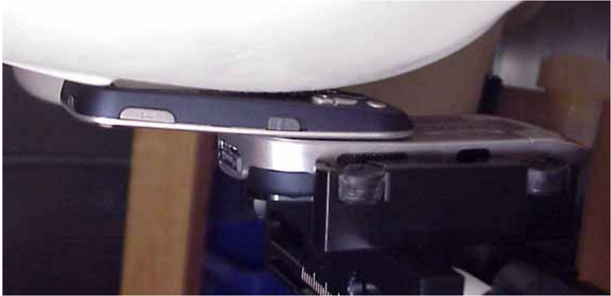
Position of device against head phantom using the “cheek” open position
