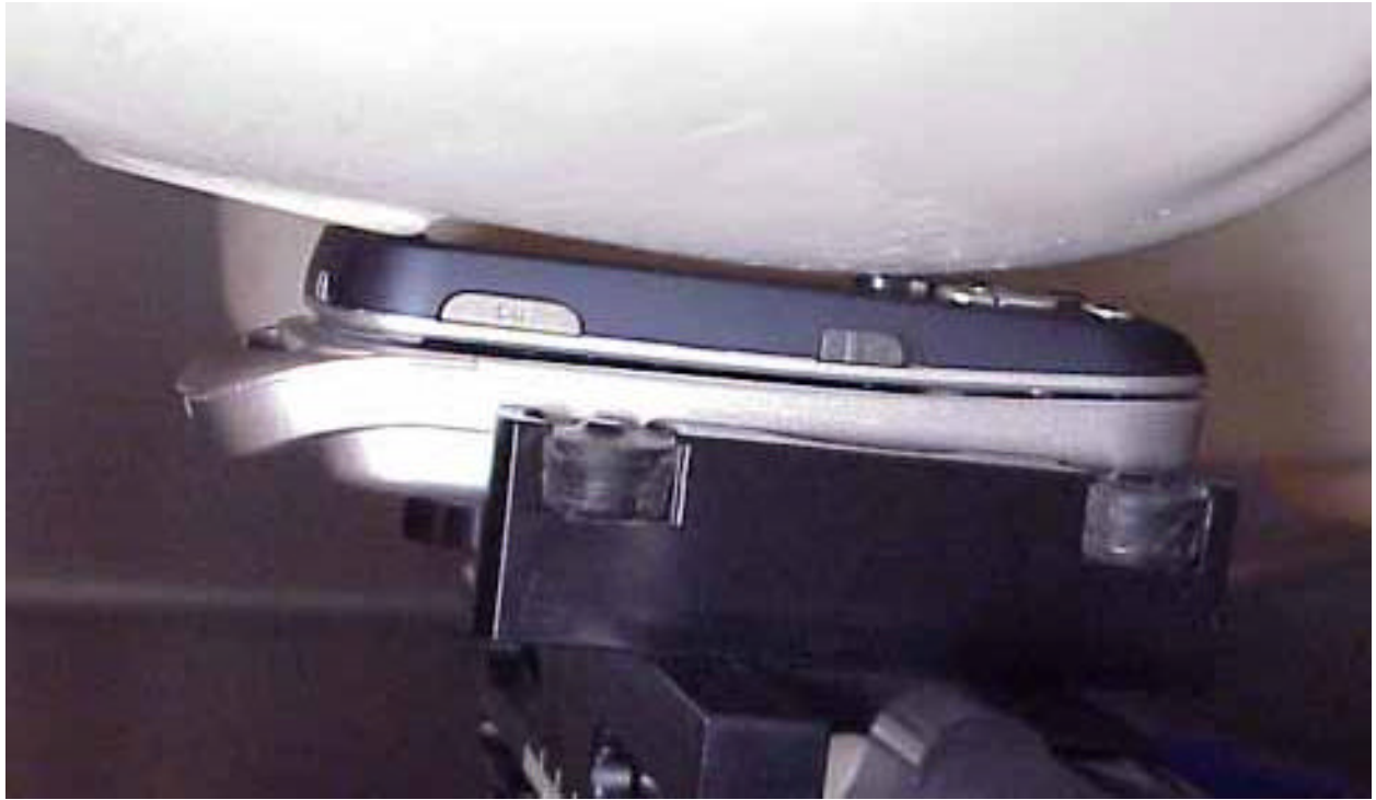
Position of device against head phantom using the “cheek” closed position
