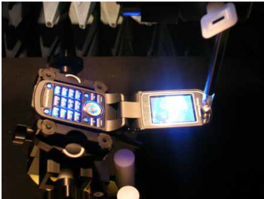
Figure 12-1 Test Setup for Wireless Device
