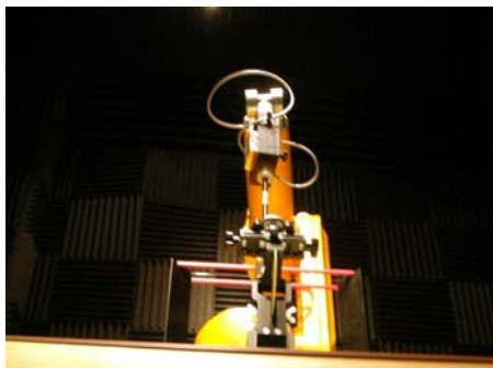
Figure 3-1 HAC RF Emissions Measurement System
