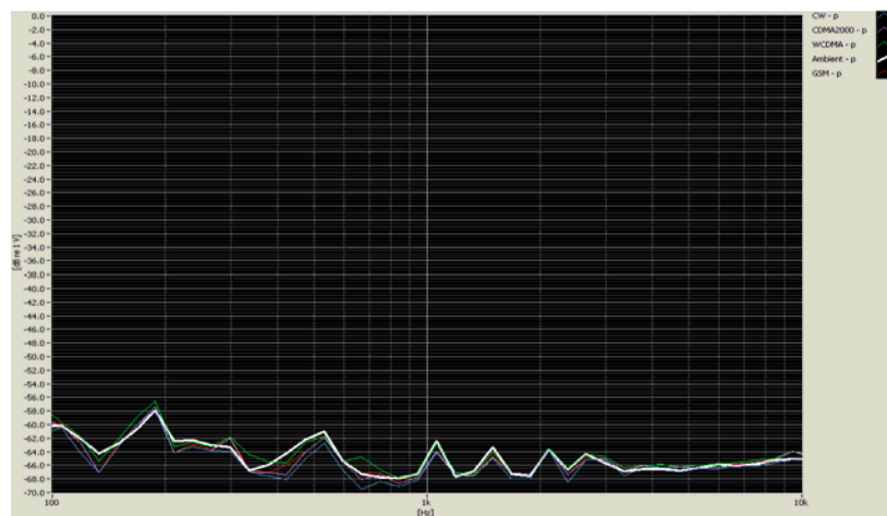
Figure 5-15 High power RF Emissions Effect with HAC Dipole on the T-coil Probe System
