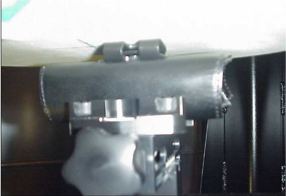
Position of device against flat phantom using carry accessory ICE-20 with hands free accessory (HPB-20).
