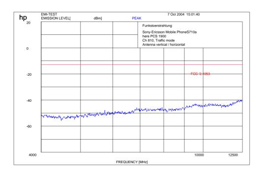
The measurements were performed up to 20 GHz with a special low-noise preamp and a wideband horn antenna. There were no spurs found.
