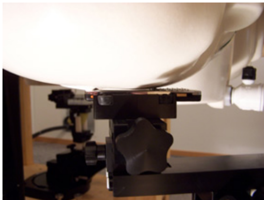
Device position against the head: Cheek (touch) phone position
