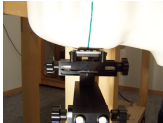
Device position against the head: Cheek (touch) phone position
