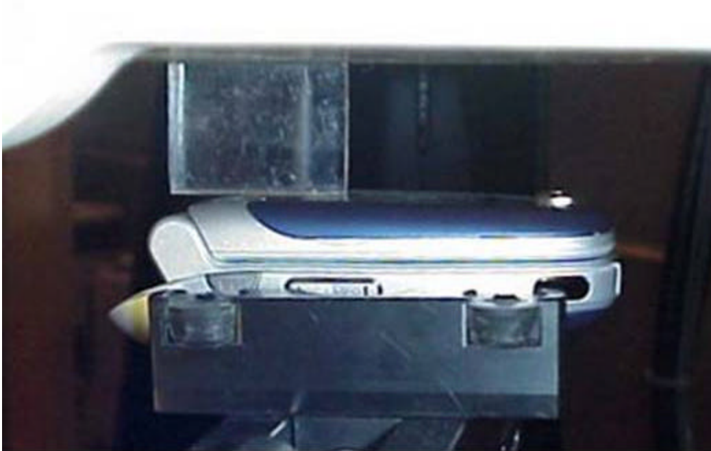
Position with front of device against flat phantom closed using a 25MM SPACER for PTT.
