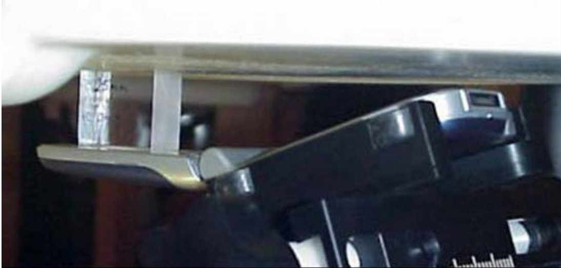
Position with front of device against flat phantom open using a 25MM SPACER for PTT.
