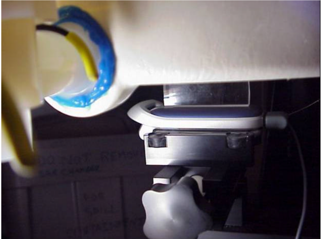
Position with back of device against flat phantom using a 20MM SPACER with hands free accessory.
