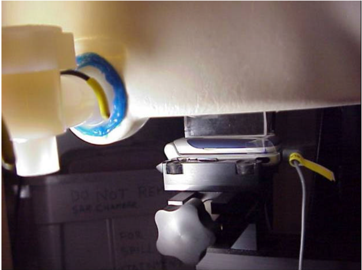
Position with front of device against flat phantom using a 20MM SPACER with hands free accessory.
