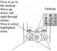
Press to go back one level in the menus. Press and hold to return to standby.
