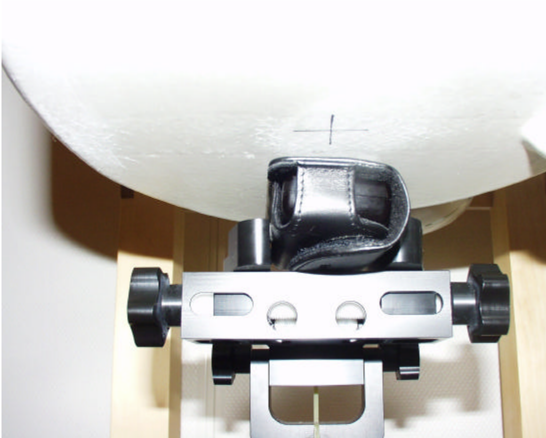
Device position against the body: Phone inside case and in touch with the flat position of phantom
