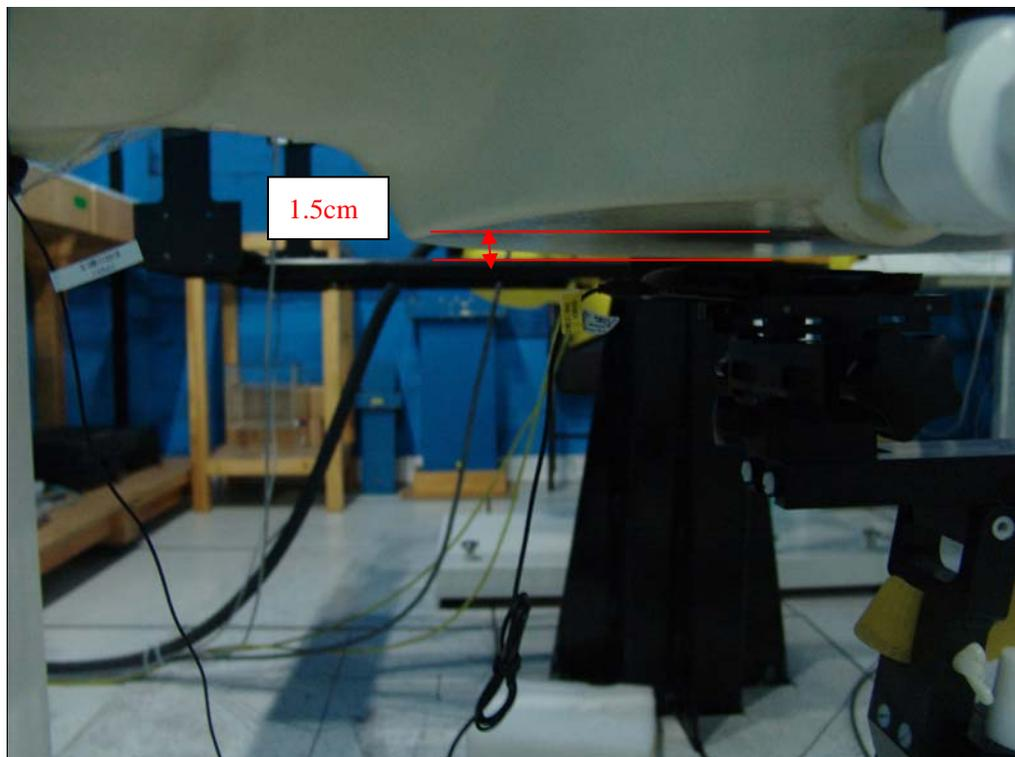
**Picture G8: Body-worn Position with Headset (towards ground, the distance from handset to the bottom of the Phantom is 1.5cm)**
