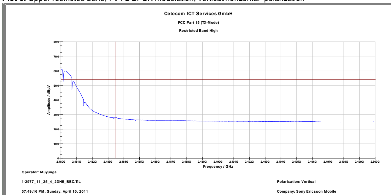
Plot 6: Upper restricted band, Pi/4 DQPSK modulation, vertical/horizontal polarization
