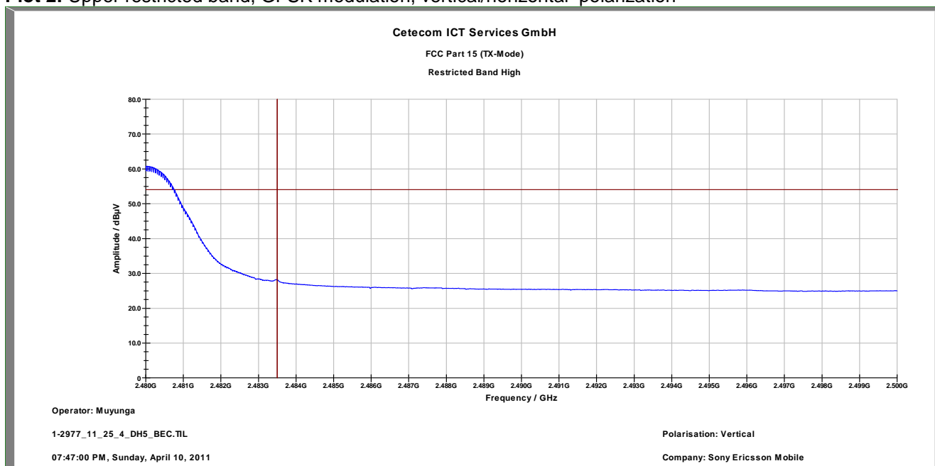
Plot 2: Upper restricted band, GFSK modulation, vertical/horizontal polarization
