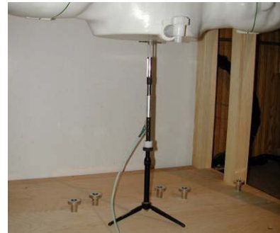
Figure 12-2 System Verification Setup Photo
