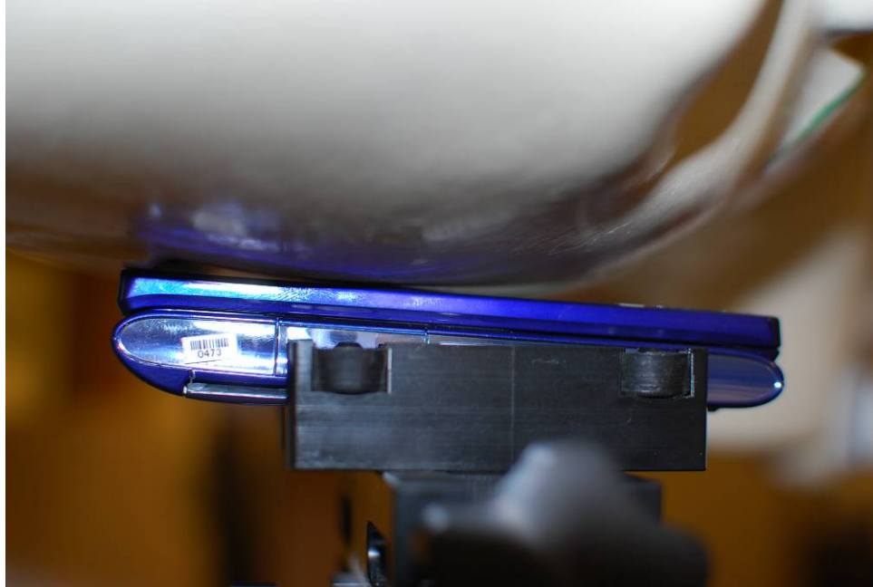
Figure 19-1 SAR Test Setup Photo 1
