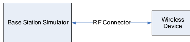
Figure 14-1 Power Measurement Setup
