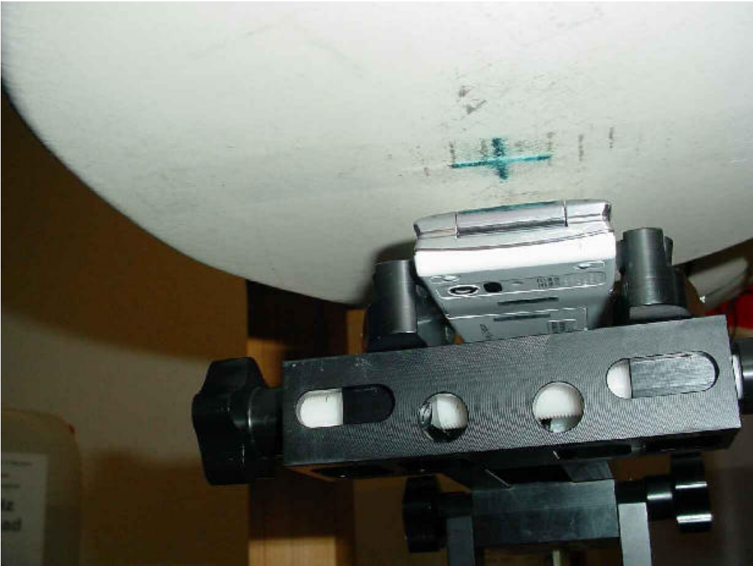
Photo 24: Test position body worn rear side (15 mm distance)
