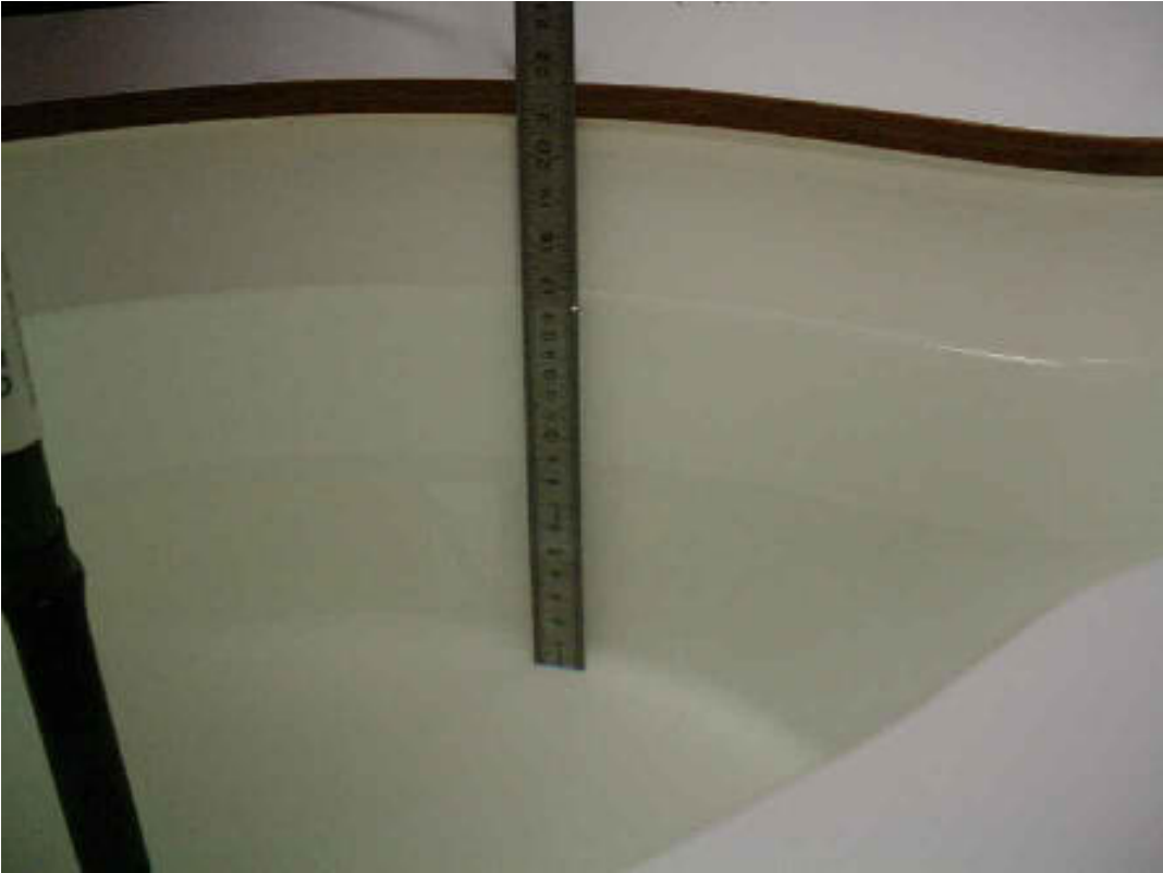
Photo 27: Liquid depth 1900 MHz body simulating liquid
