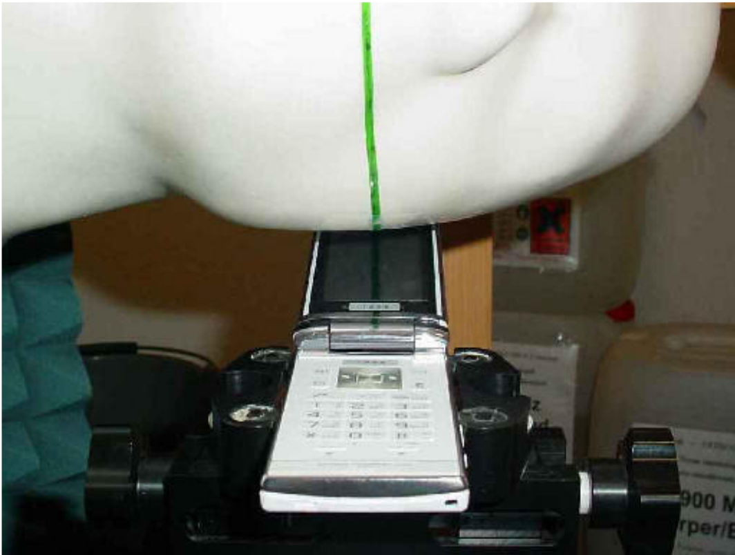
Photo 16: Test position left hand tilted 15°
