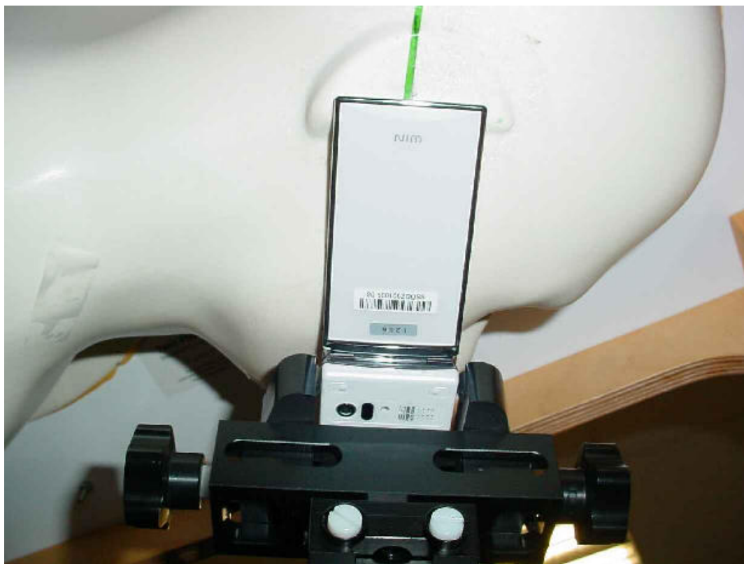
Photo 20: Test position right hand tilted 15°
