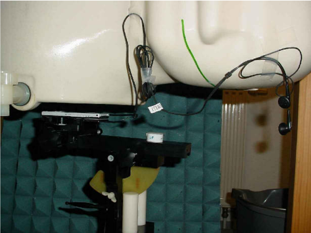
Photo 24: Test position body worn rear side (15 mm distance)
