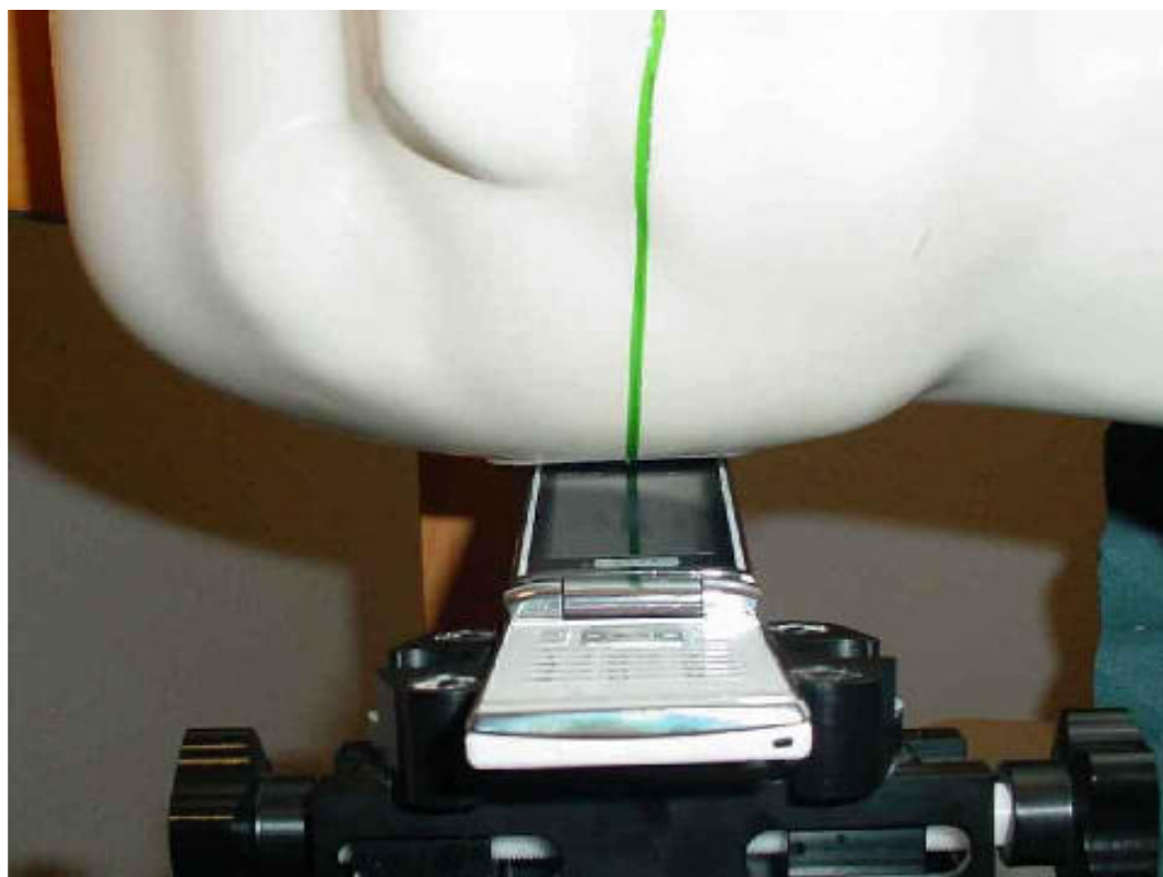
Photo 20: Test position right hand tilted 15°
