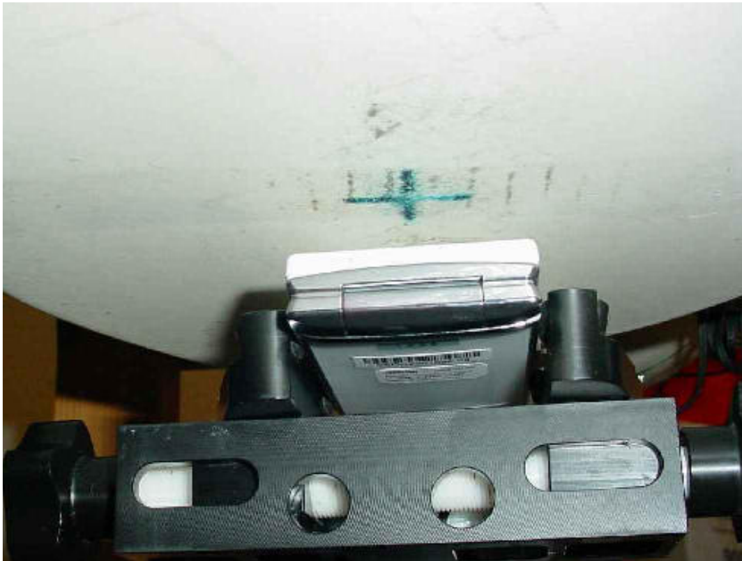
Photo 25: Test position body worn rear side (15 mm distance)
