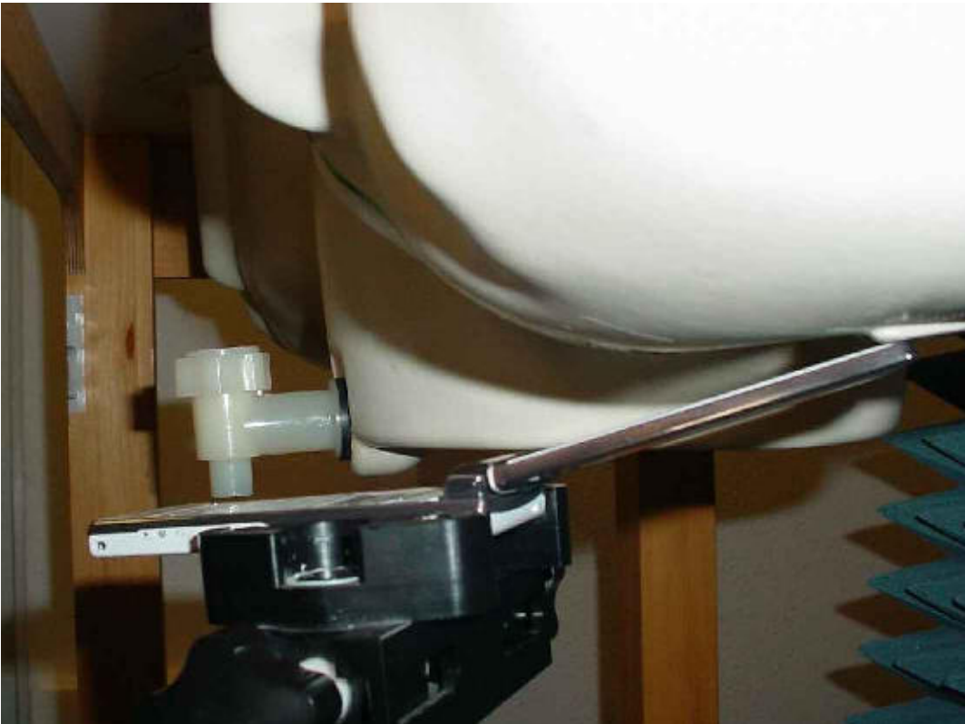
Photo 16: Test position left hand tilted 15°
