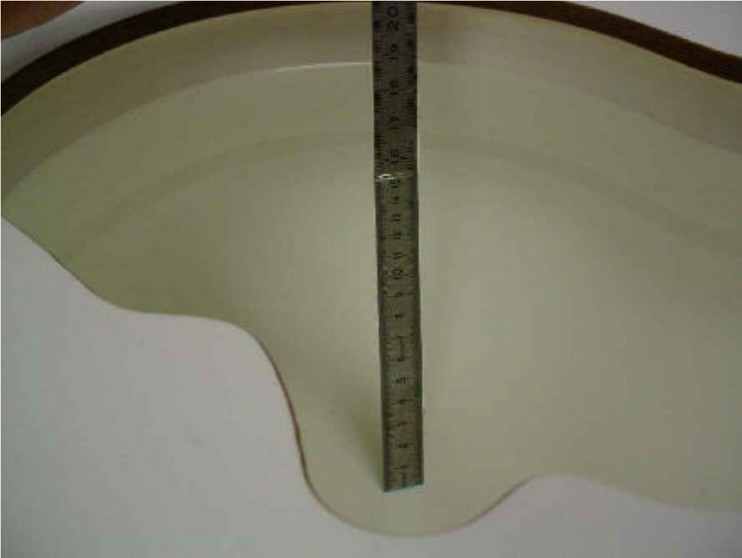
Photo 27: Liquid depth 1900 MHz body simulating liquid
