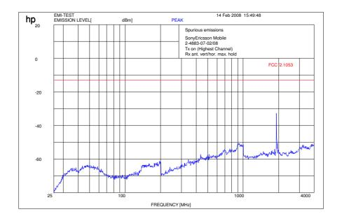
Carrier suppressed with a rejection filter
