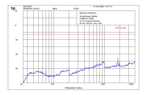
Carrier suppressed with a rejection filter
