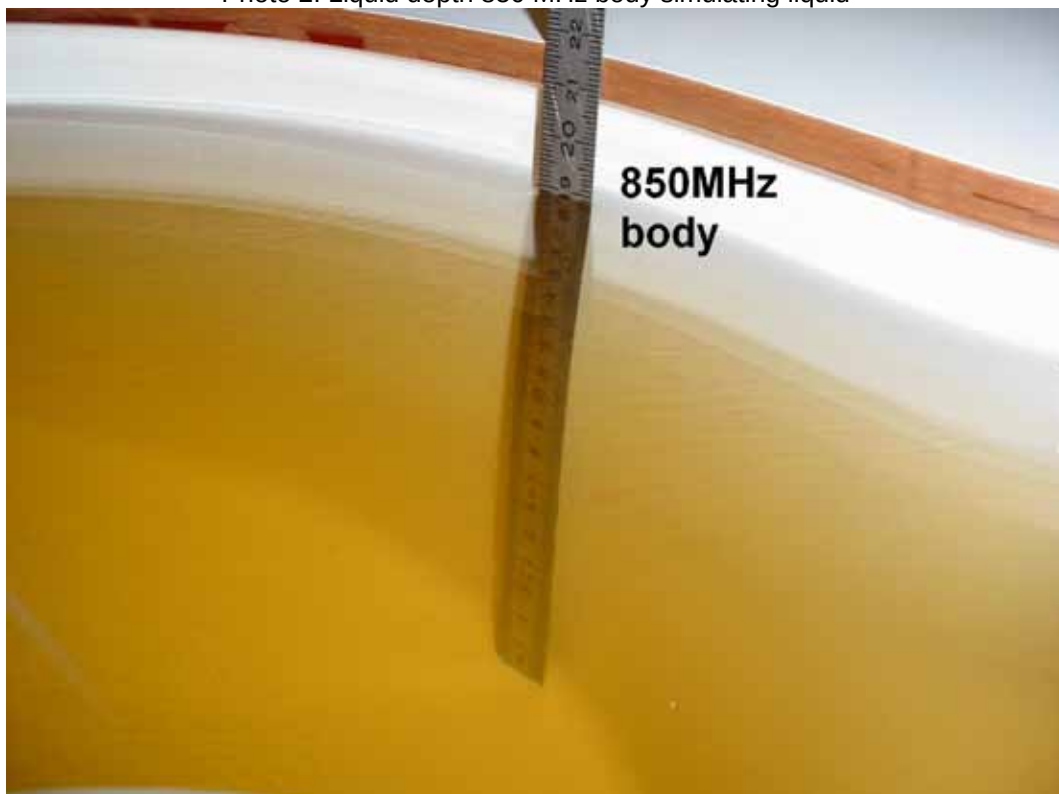
Photo 2: Liquid depth 850 MHz body simulating liquid
