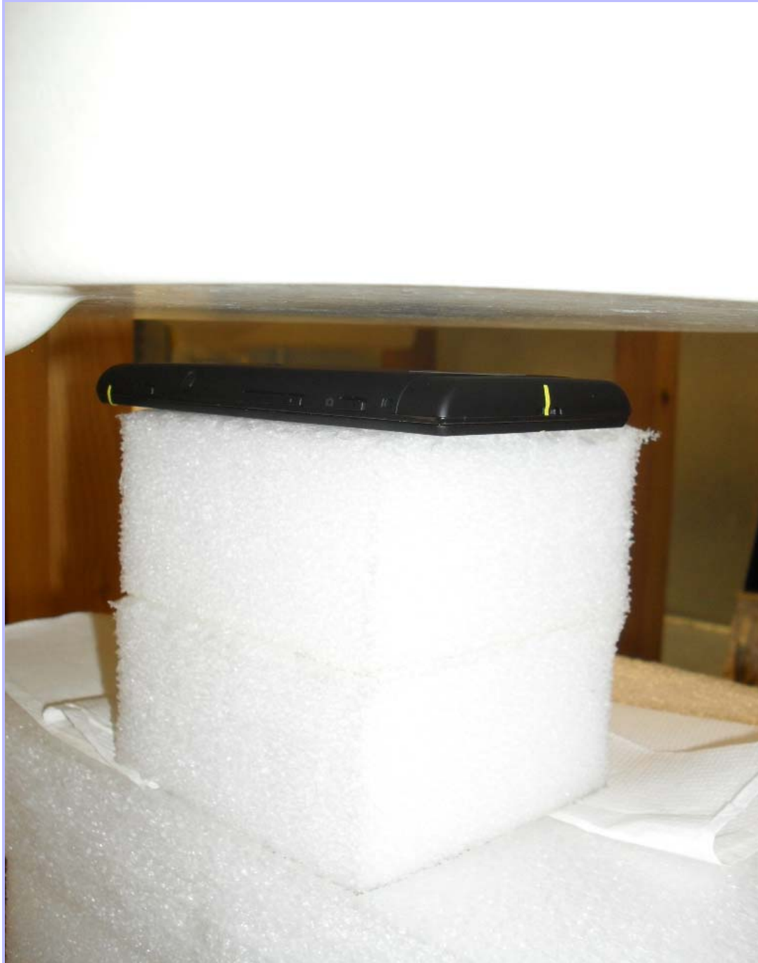
PHT/85123JD01/009: Rear of EUT Facing Phantom at 15mm separation
