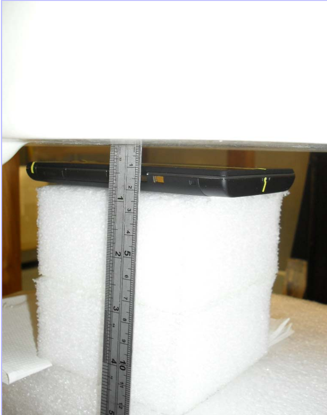
PHT/85123JD01/006: Front of EUT Facing Phantom at 10mm separation
