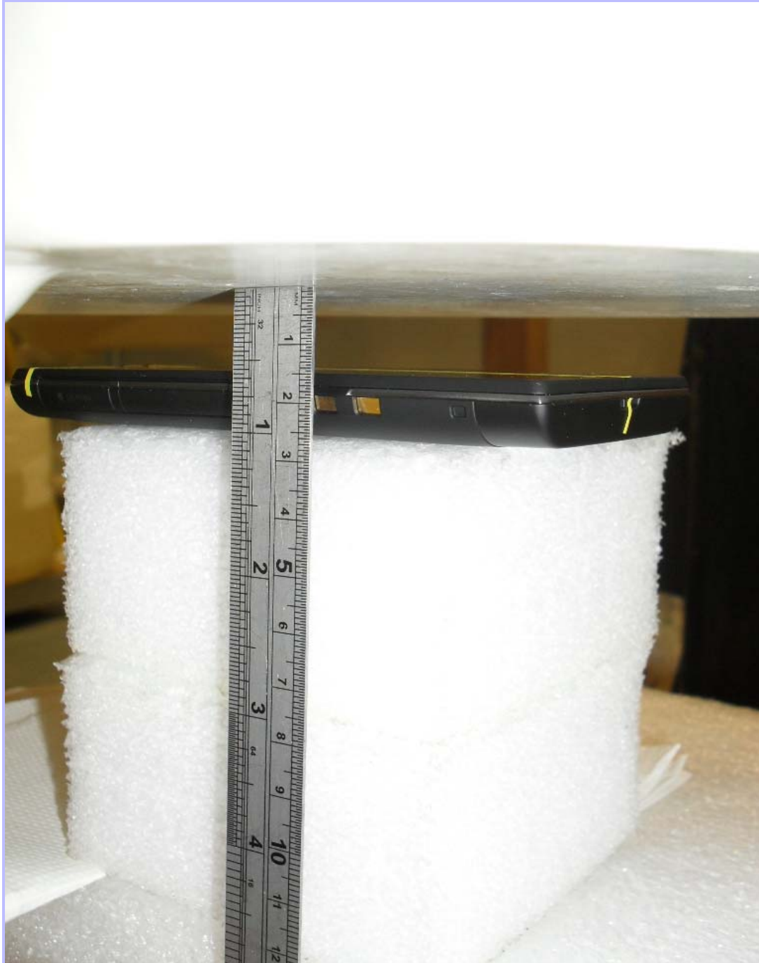
PHT/85123JD01/007: Front of EUT Facing Phantom at 15mm separation
