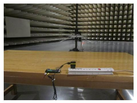
**Layout of AC Powerline Conducted Emission**
