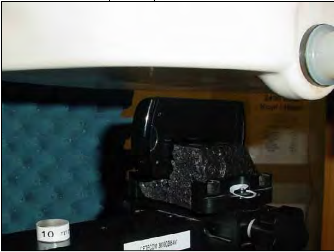
Photo 22: Test position body worn right side with 10mm distance
