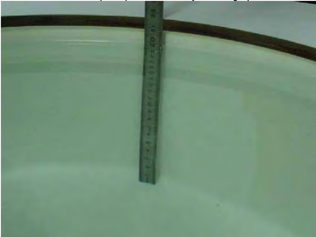
Photo 4: Liquid depth 1900 MHz body simulating liquid
