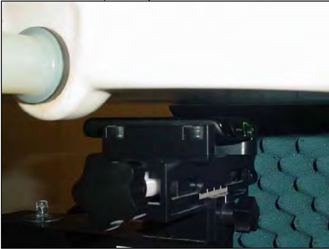
Photo 20: Test position body worn rear side with 10mm distance
