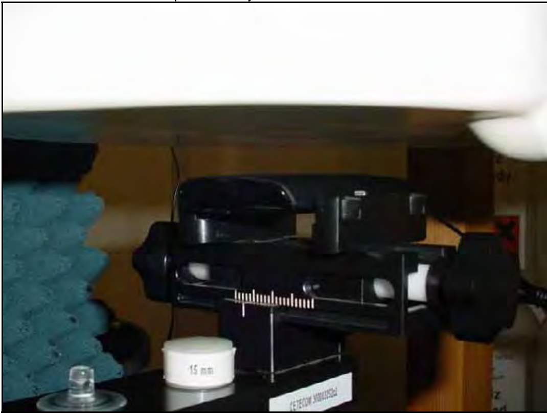
Photo 25: Test position body worn rear side with 15mm distance
