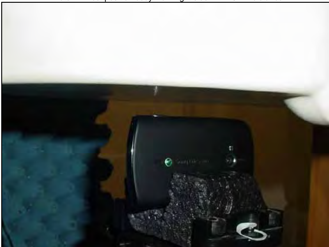
Photo 22: Test position body worn right side with 10mm distance
