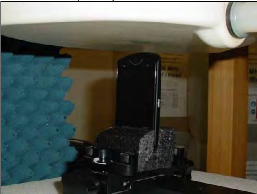
Photo 24: Test position body worn bottom side with 10mm distance
