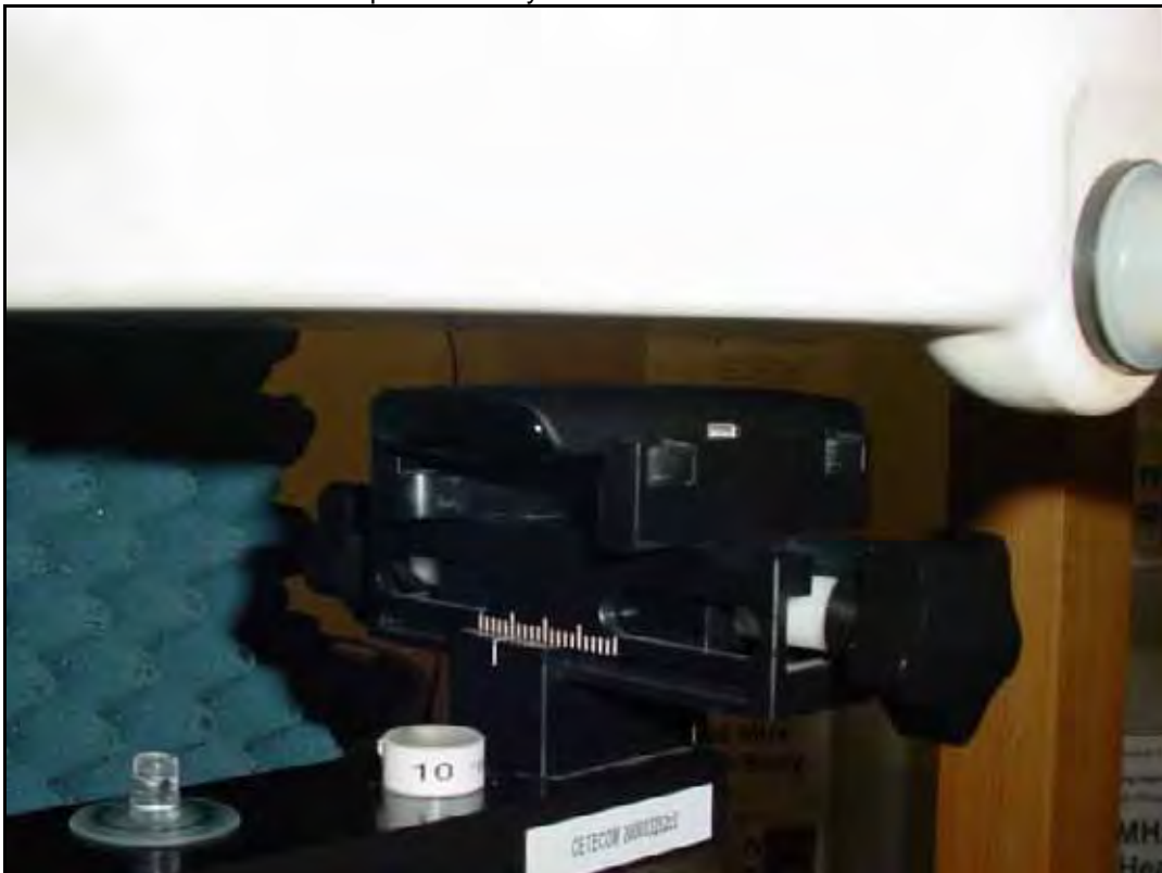
Photo 20: Test position body worn rear side with 10mm distance
