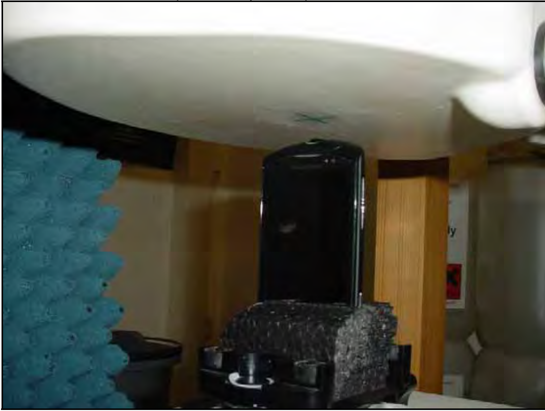
Photo 24: Test position body worn bottom side with 10mm distance
