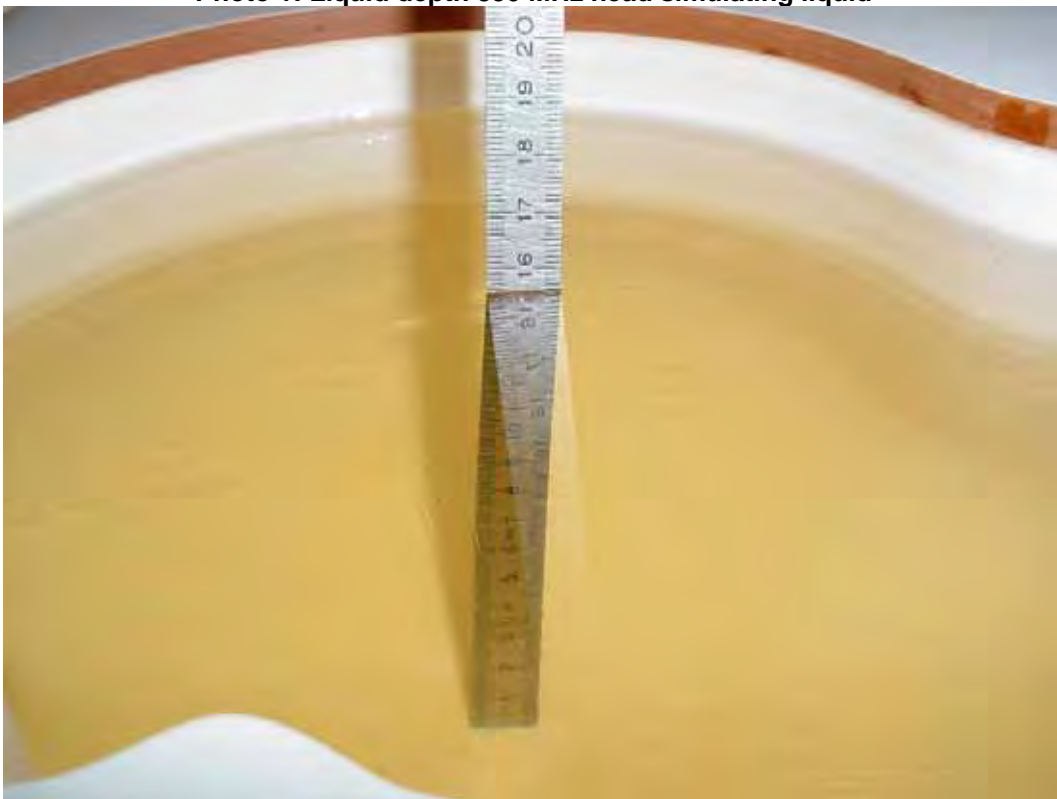
Photo 2: Liquid depth 850 MHz body simulating liquid
