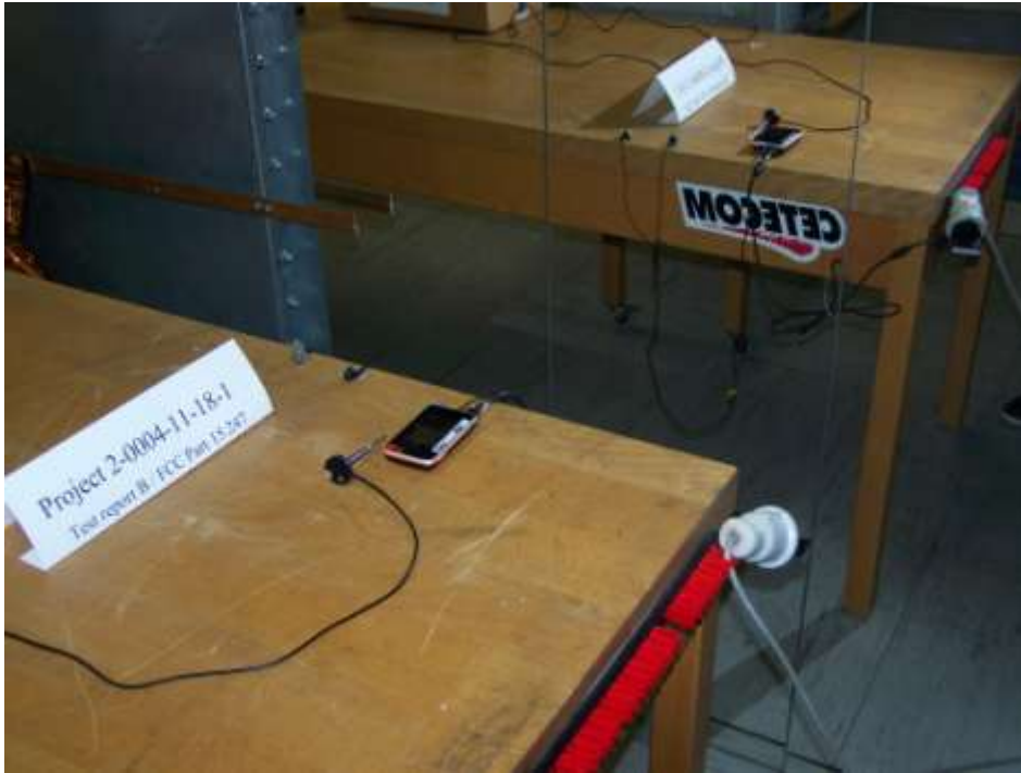
Photograph 3: Conducted test set-up, emissions on AC-mains
