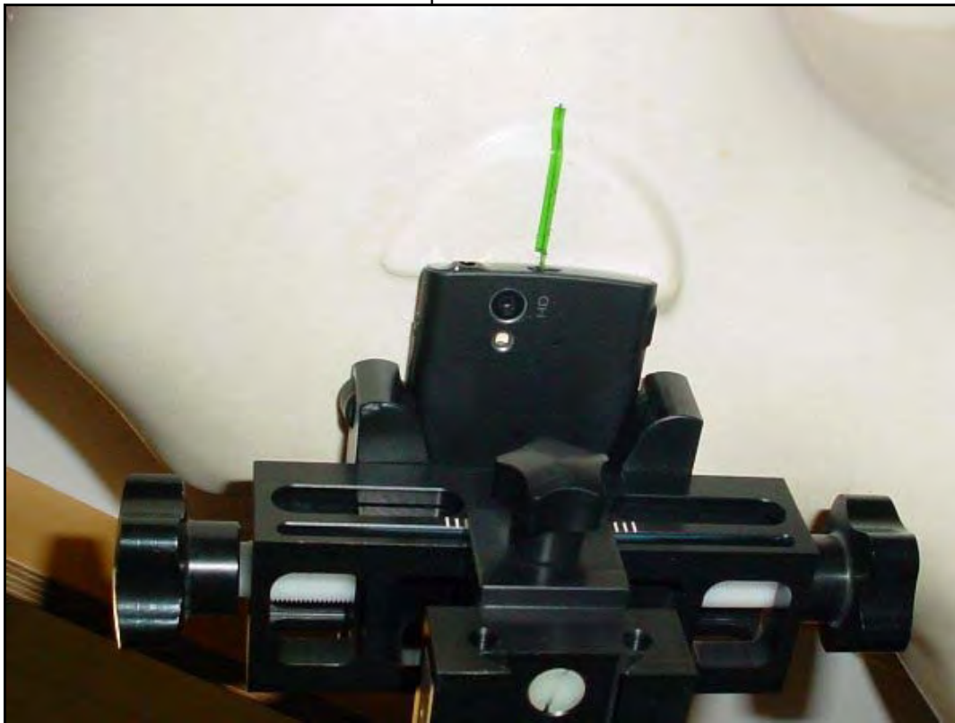
Photo 12: Test position left hand tilted 15°
