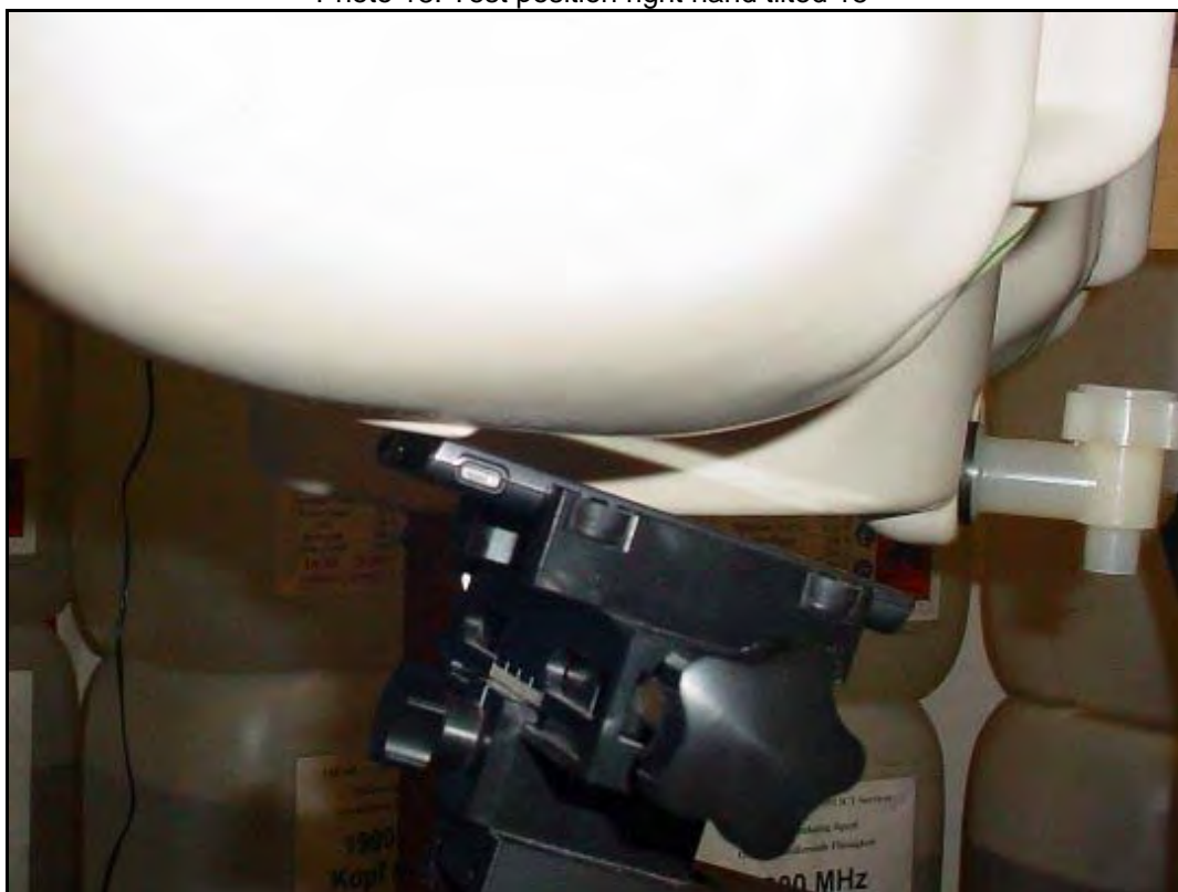
Photo 18: Test position right hand tilted 15°
