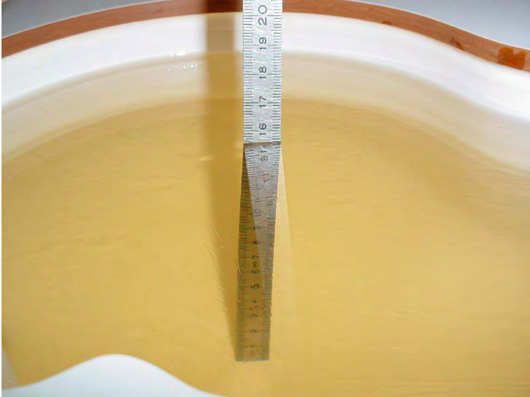
Photo 2: Liquid depth 850 MHz body simulating liquid
