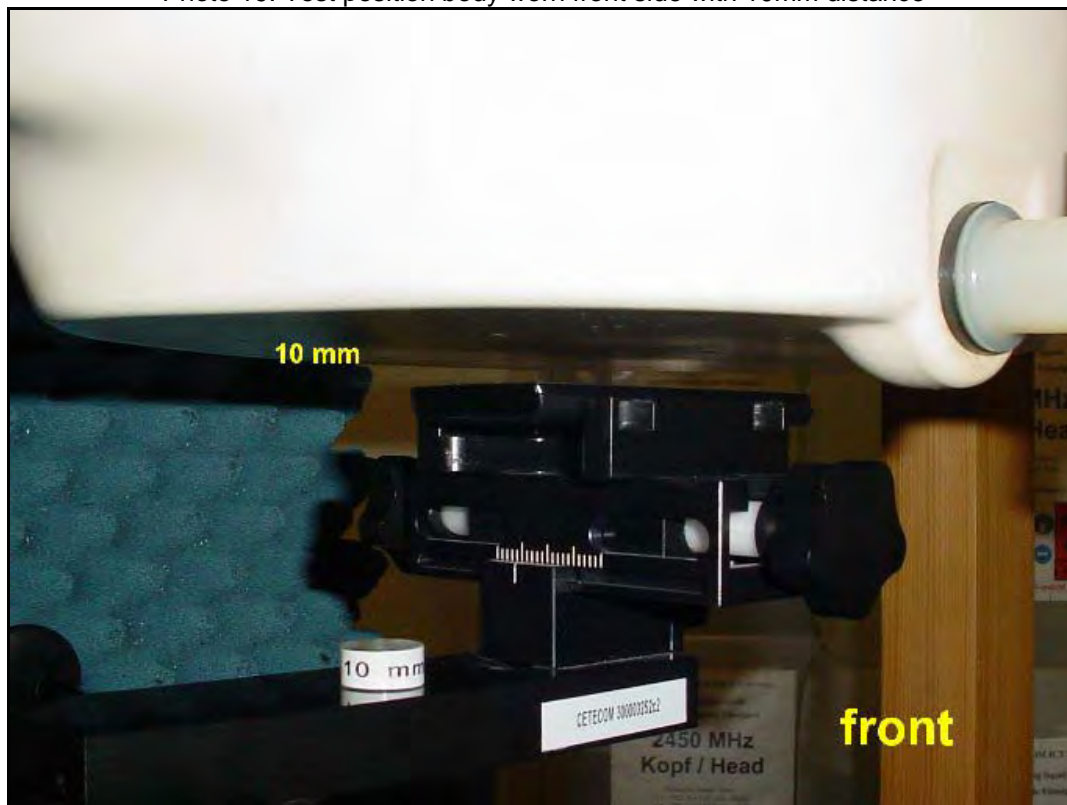
Photo 20: Test position body worn left edge side with 10mm distance
