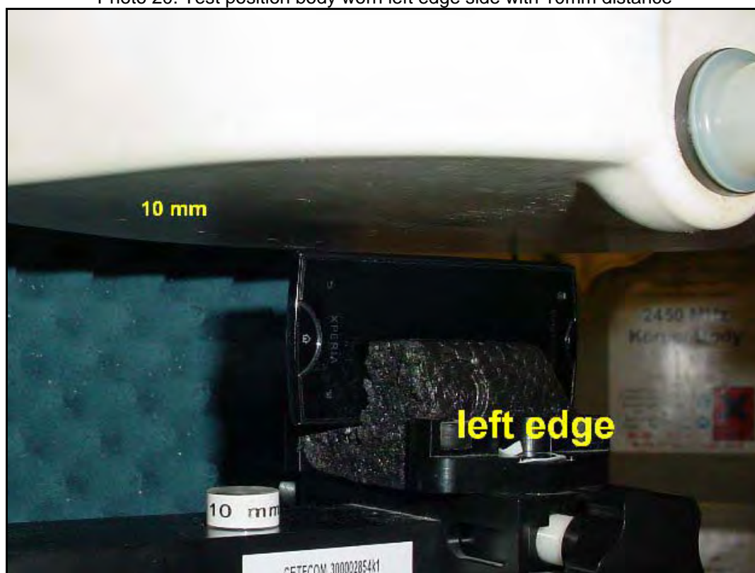
Photo 20: Test position body worn left edge side with 10mm distance
