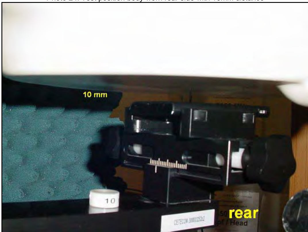
Photo 24: Test position body worn rear side with 10mm distance
