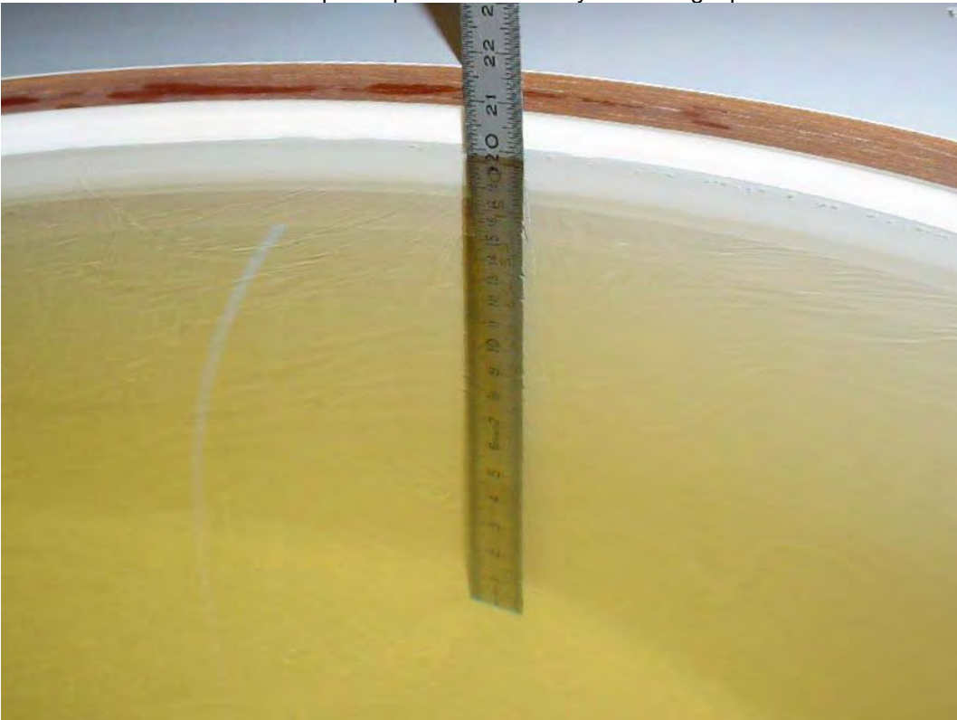
Photo 2: Liquid depth 850 MHz body simulating liquid
