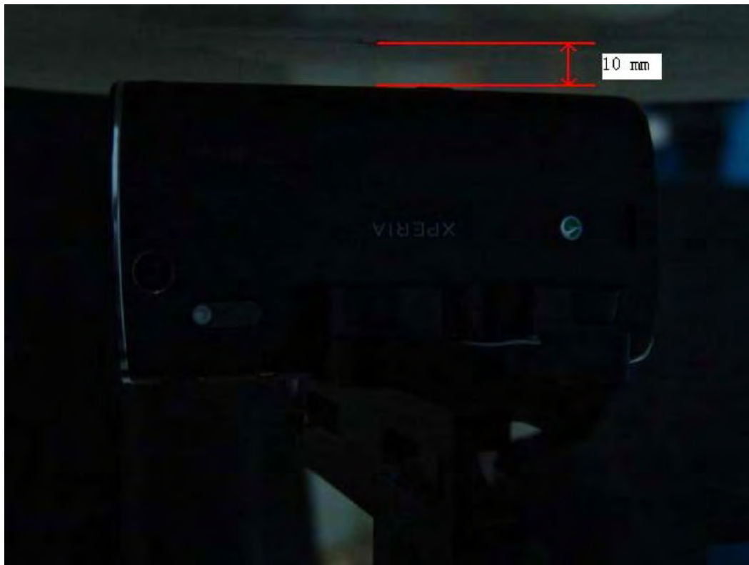
Picture G10: Body-worn Position (EUT'left side towards phantom, the distance from handset to the bottom of the Phantom is 10 mm)
