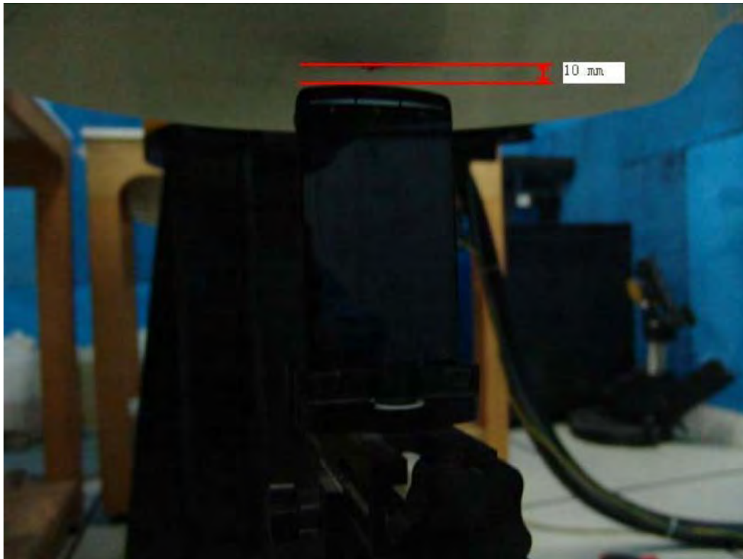
Picture G11: Body-worn Position (EUT's bottom side towards phantom, the distance from handset to the bottom of the Phantom is 10 mm)
