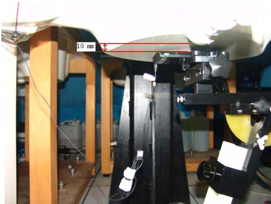
Picture G8: Body-worn Position with Headset (EUT towards ground, the distance from handset to the bottom of the Phantom is 10 mm)
