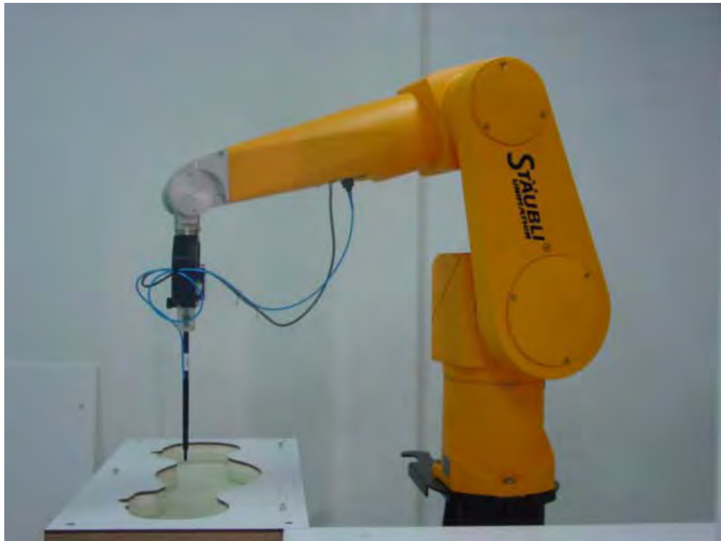
Picture B1: Specific Absorption Rate Test Layout
