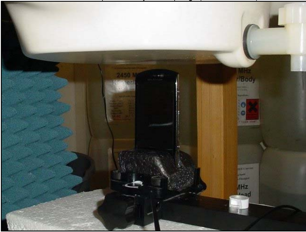
Photo 24: Test position body worn bottom edge (10 mm distance)
