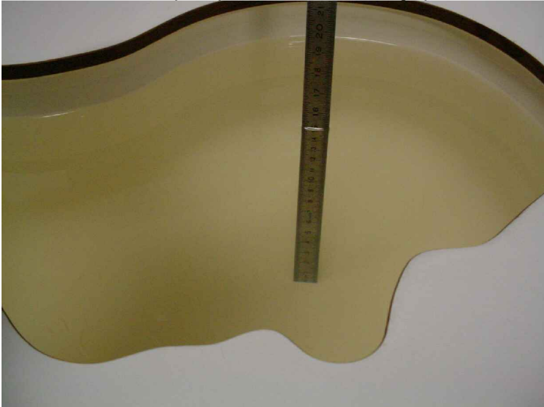
Photo 6: Liquid depth 2450 MHz body simulating liquid
