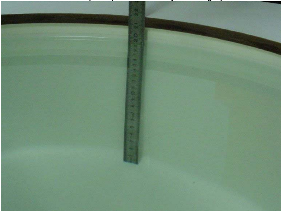
Photo 4: Liquid depth 1900 MHz body simulating liquid
