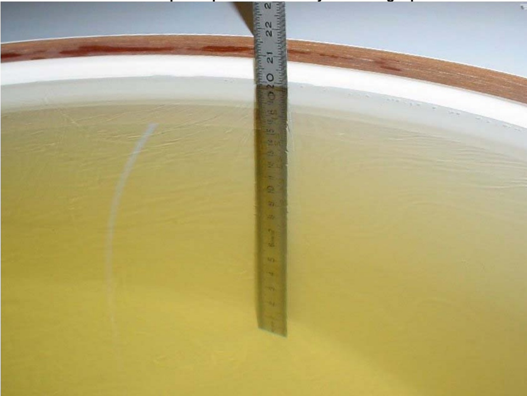
Photo 2: Liquid depth 850 MHz body simulating liquid
