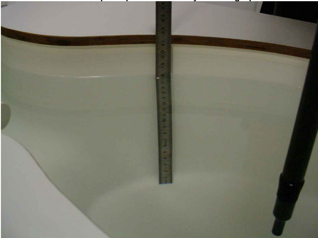
Photo 6: Liquid depth 2450 MHz body simulating liquid
