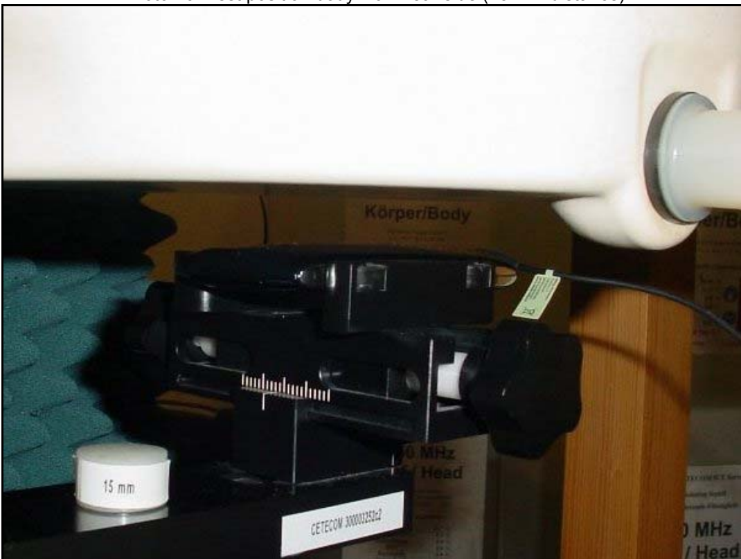
Photo 26: Test position body worn rear side (15 mm distance)
