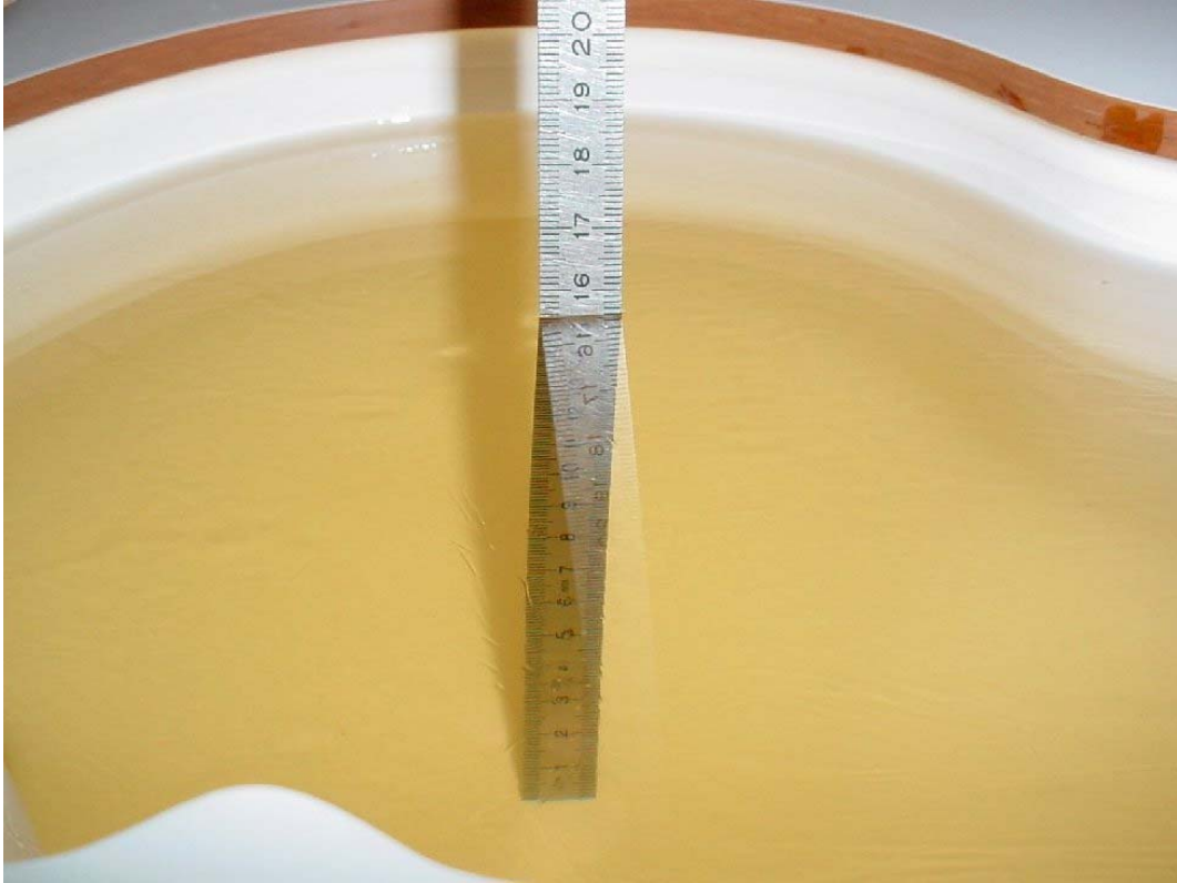
Photo 2: Liquid depth 850 MHz body simulating liquid
