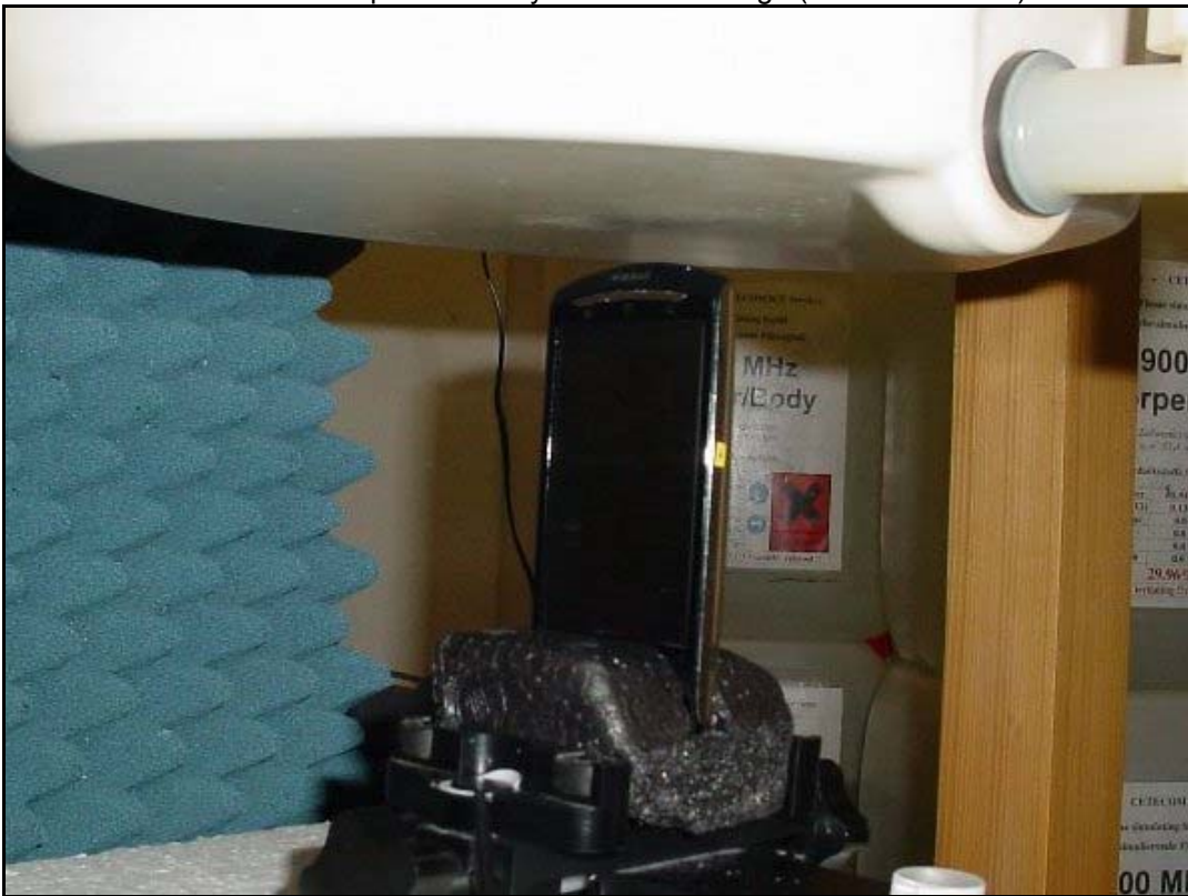
Photo 24: Test position body worn bottom edge (10 mm distance)
