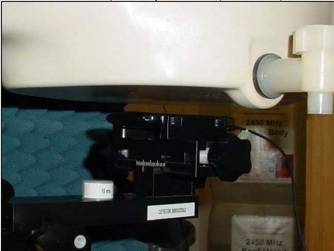
Photo 26: Test position body worn rear side (15 mm distance)
