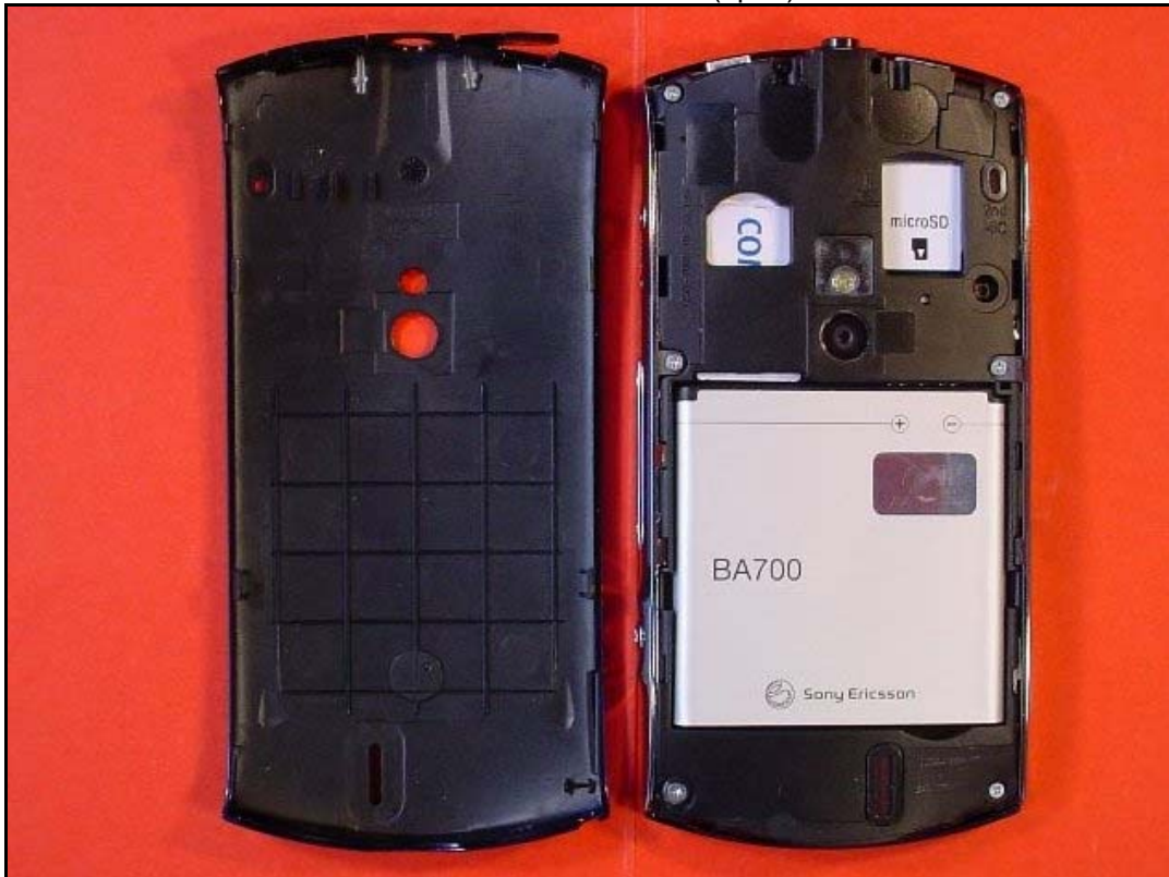
Photo 6: DUT - rear view (open) without battery
