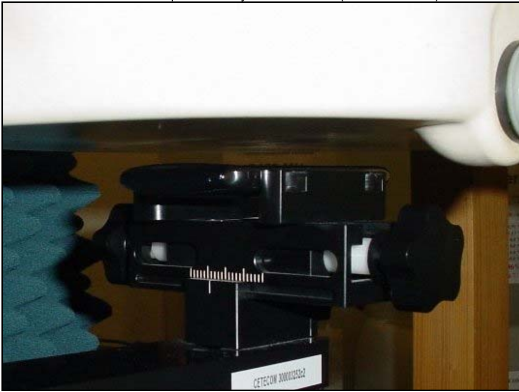
Photo 20: Test position body worn rear side (10 mm distance)
