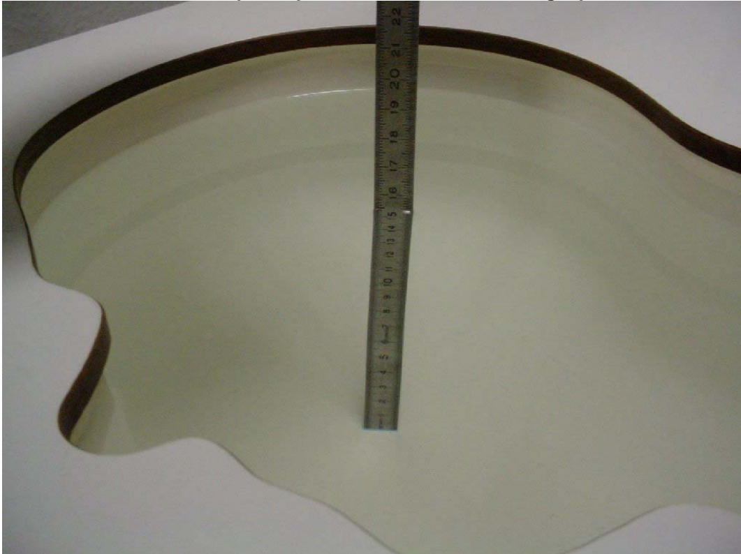
Photo 4: Liquid depth 1900 MHz body simulating liquid
