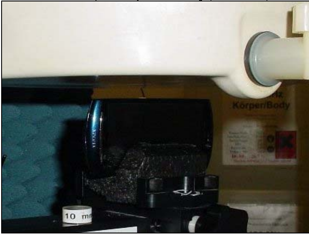
Photo 22: Test position body worn right side edge (10 mm distance)
