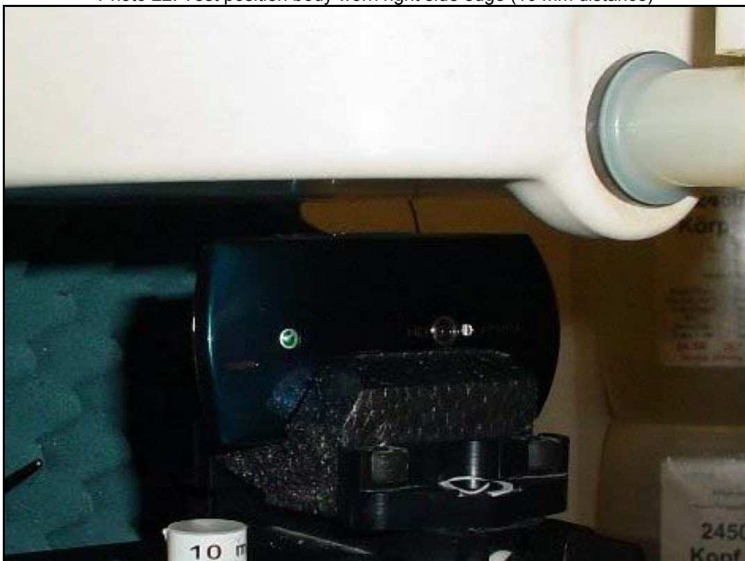
Photo 22: Test position body worn right side edge (10 mm distance)
