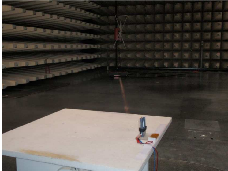
Photo 4: radiated measurements lower 1GHz
