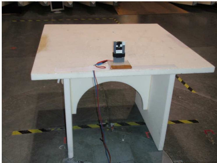
Photo 5: radiated measurements lower 1GHz
