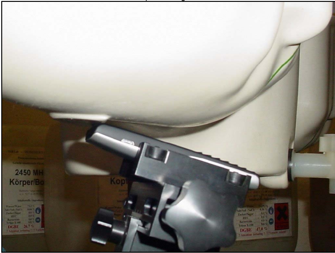
Photo 18: Test position body worn front side with 15 mm distance
