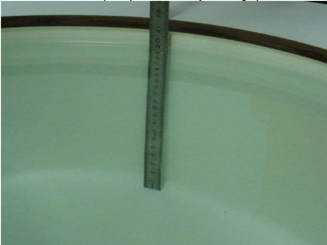
Photo 4: Liquid depth 1900 MHz body simulating liquid
