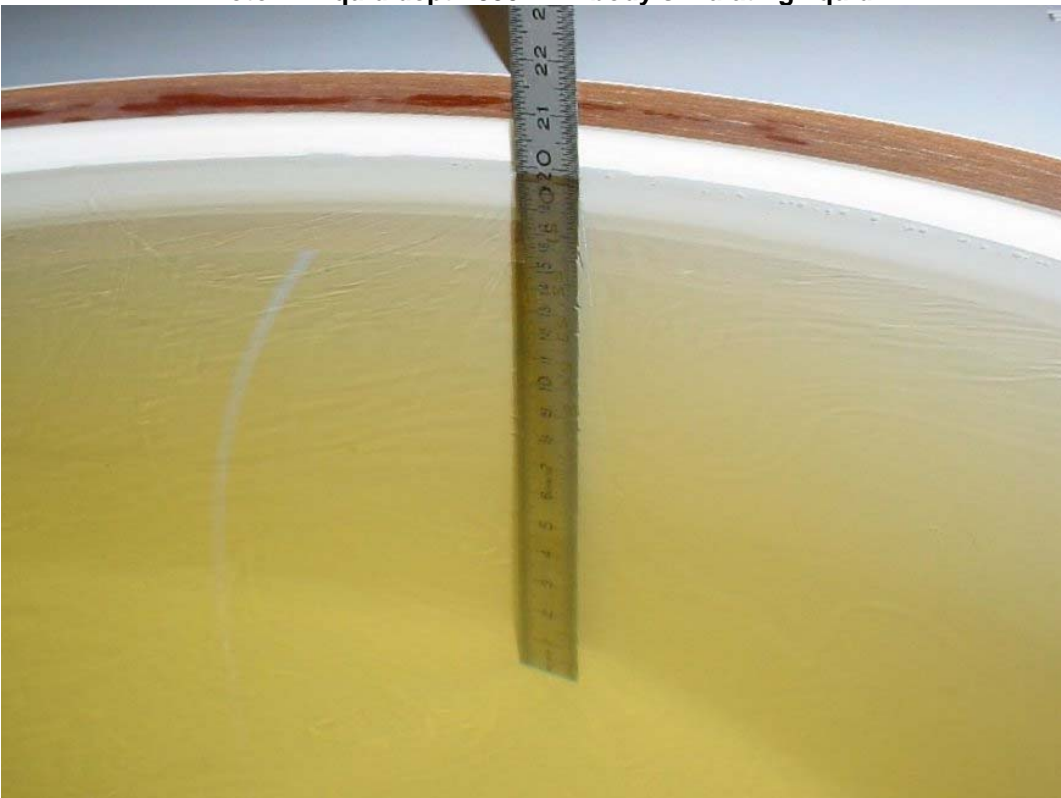
Photo 2: Liquid depth 850 MHz body simulating liquid
