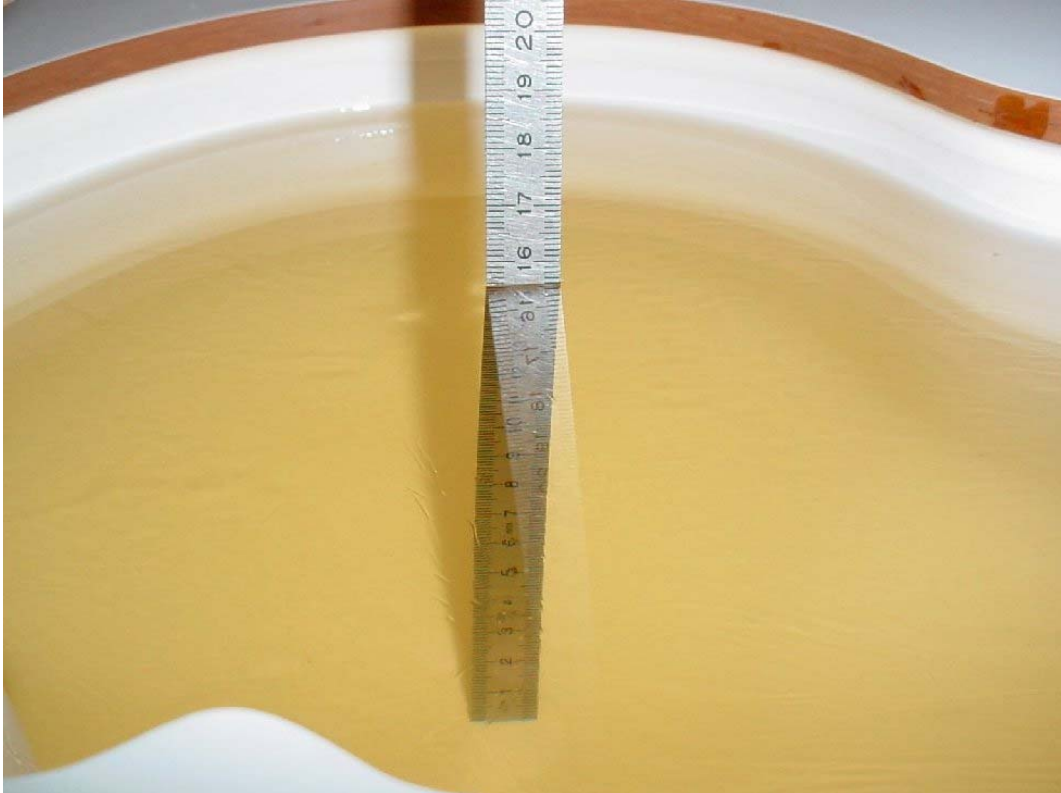
Photo 2: Liquid depth 850 MHz body simulating liquid
