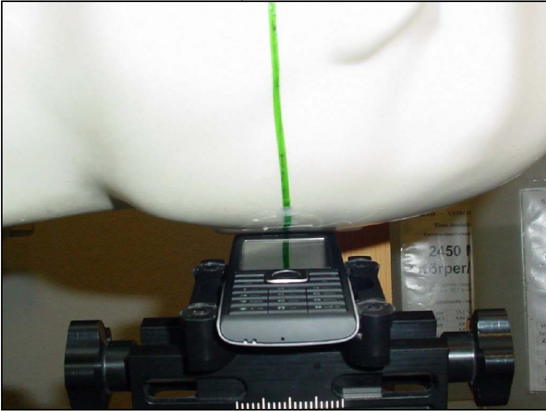
Photo 12: Test position left hand tilted 15°
