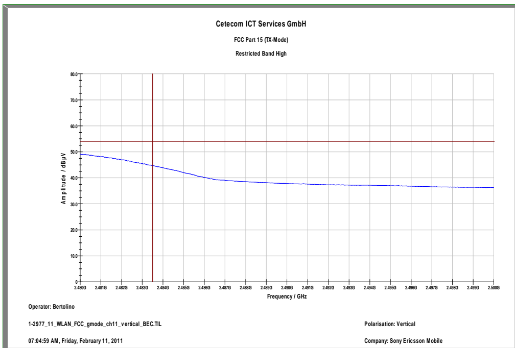
Plot 6: TX mode, upper band edge, vertical polarization
