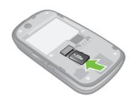
• Remove the battery cover and insert the memory card with the gold-coloured contacts facing down
