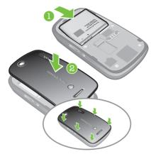
1 Insert the battery with the label side up and the 2 Attach the battery cover.
