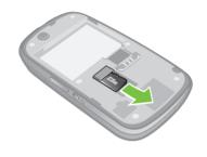
• Remove the battery cover and slide the memory card to remove it.
