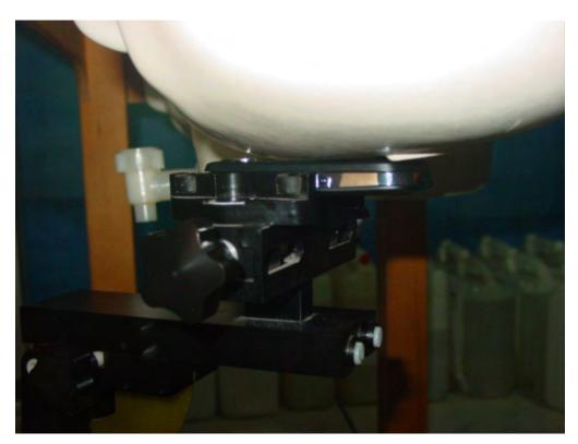
Picture G2: Left Hand Touch Cheek Position – Slide down
