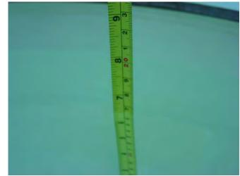
Picture B3: Liquid depth in the Flat Phantom (1900MHz Head)
