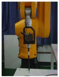
Picture3:ES3DV3 E-field probe
