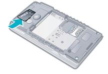
Remove the battery cover and insert the memory card with the gold-coloured contacts facing down.
