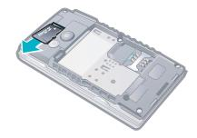
Remove the battery cover and slide the memory card to remove it.
