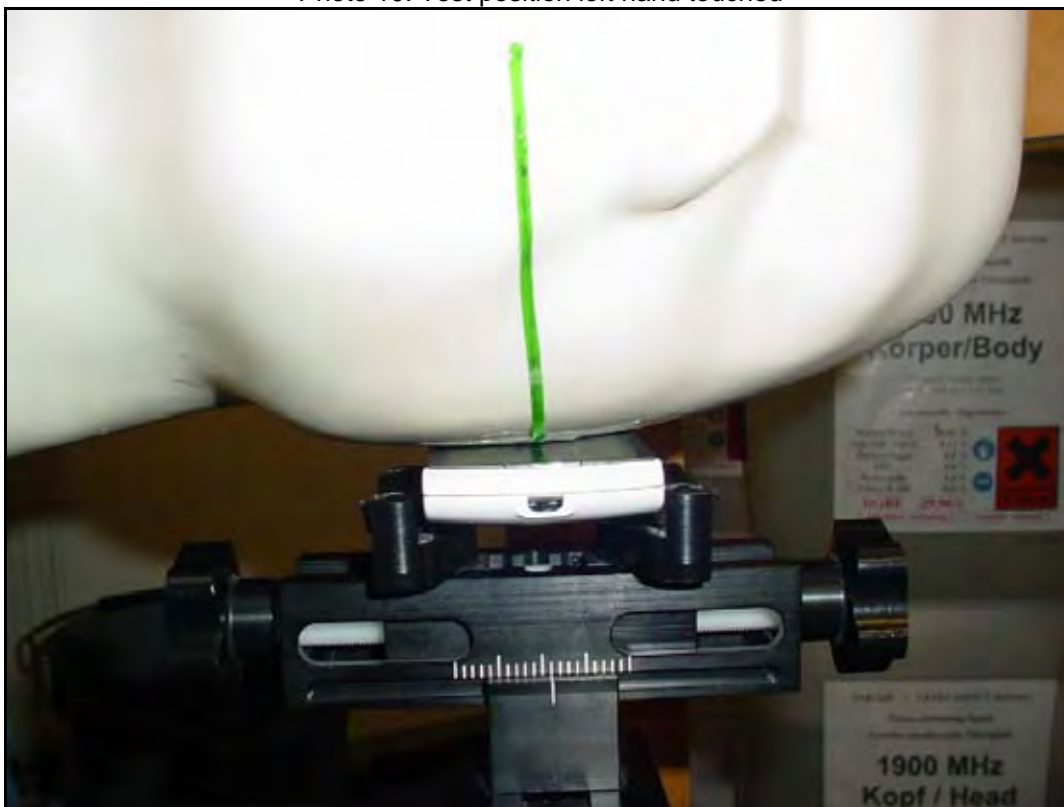
Photo 10: Test position left hand touched
