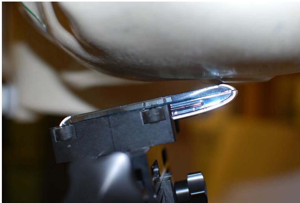
Figure 19-4 SAR Test Setup Photo 4
