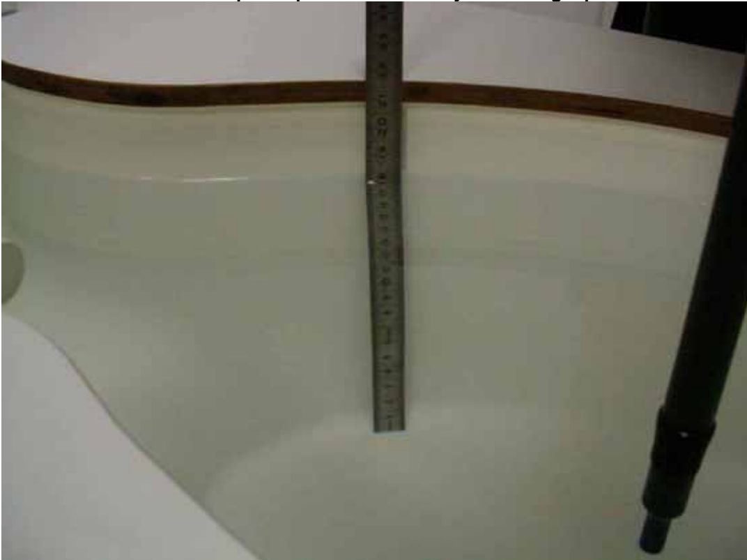
Photo 6: Liquid depth 2450 MHz body simulating liquid
