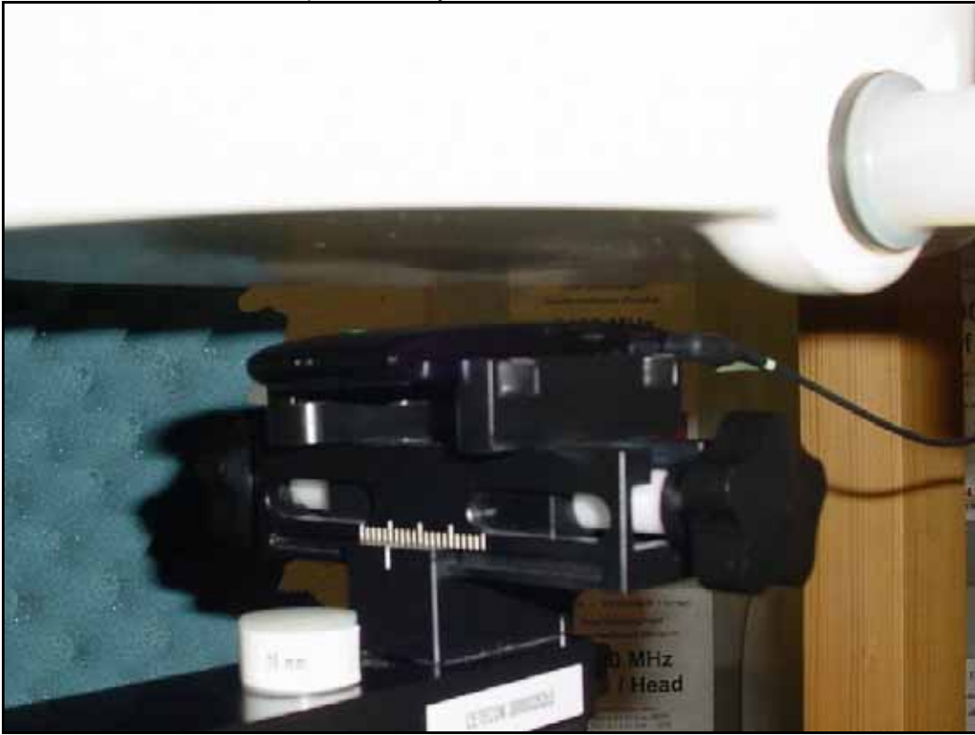
Photo 19: Test position body worn rear side with 15 mm distance
