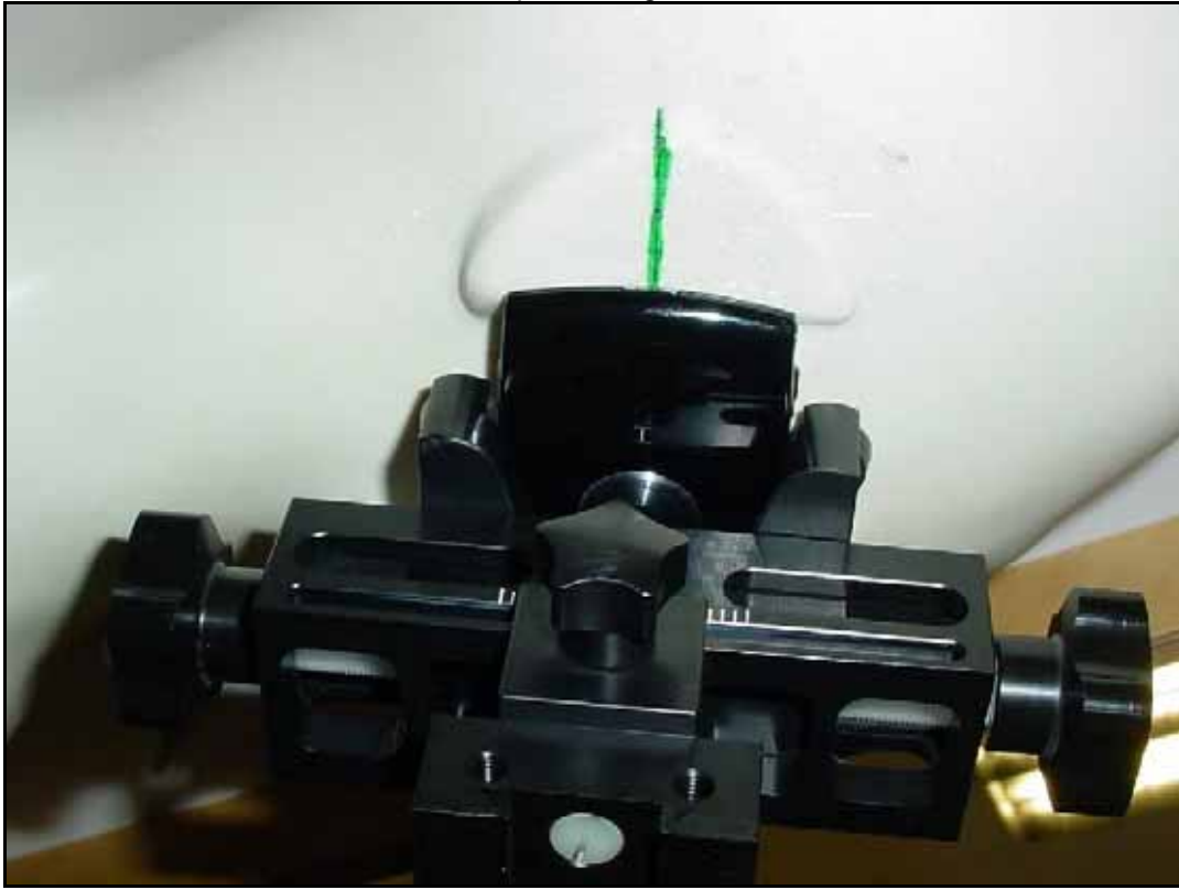
Photo 16: Test position right hand tilted 15°
