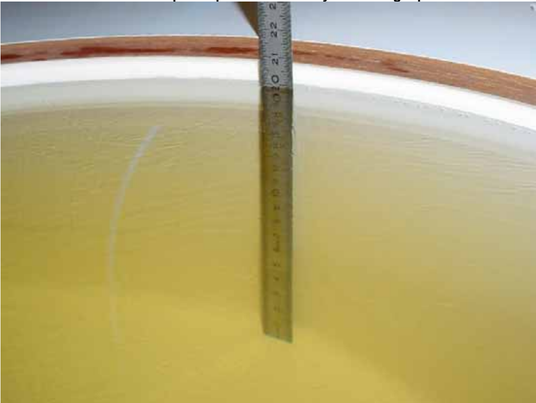
Photo 2: Liquid depth 850 MHz body simulating liquid
