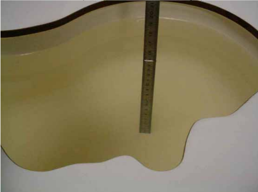
Photo 6: Liquid depth 2450 MHz body simulating liquid
