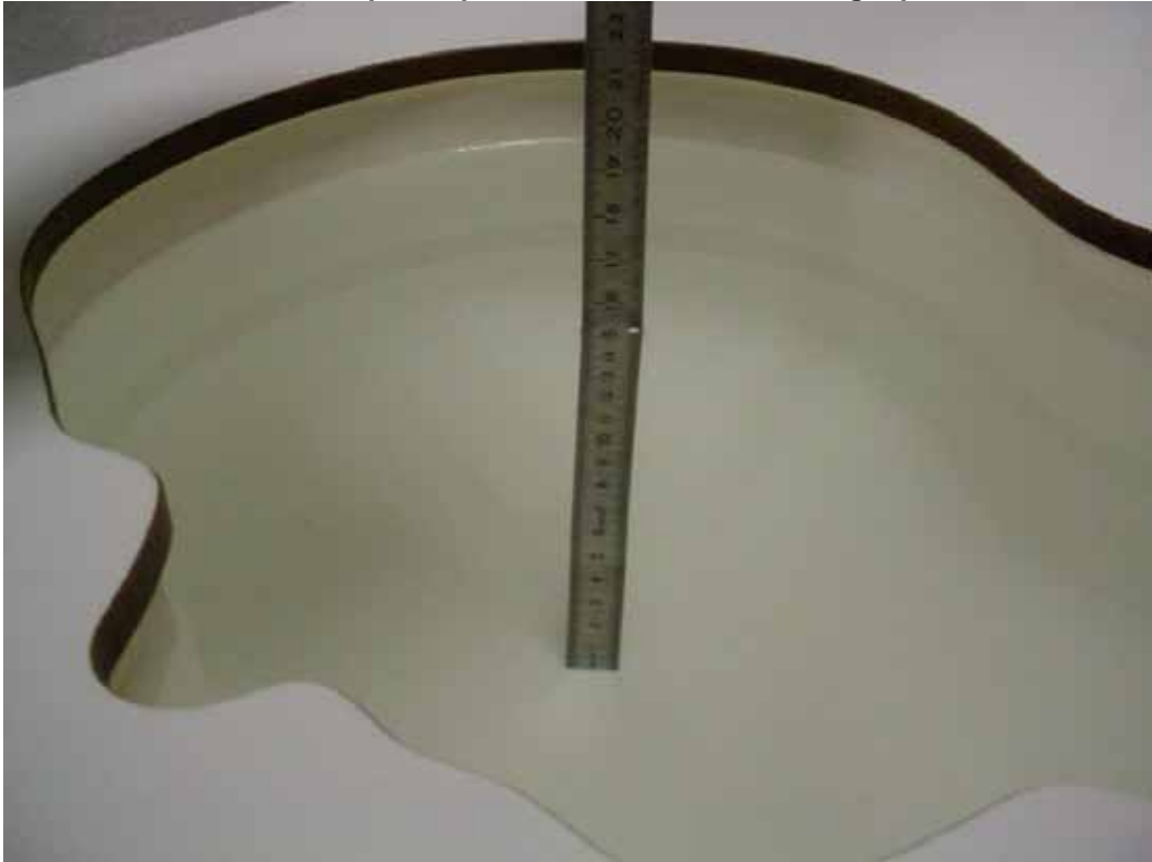
Photo 4: Liquid depth 1900 MHz body simulating liquid
