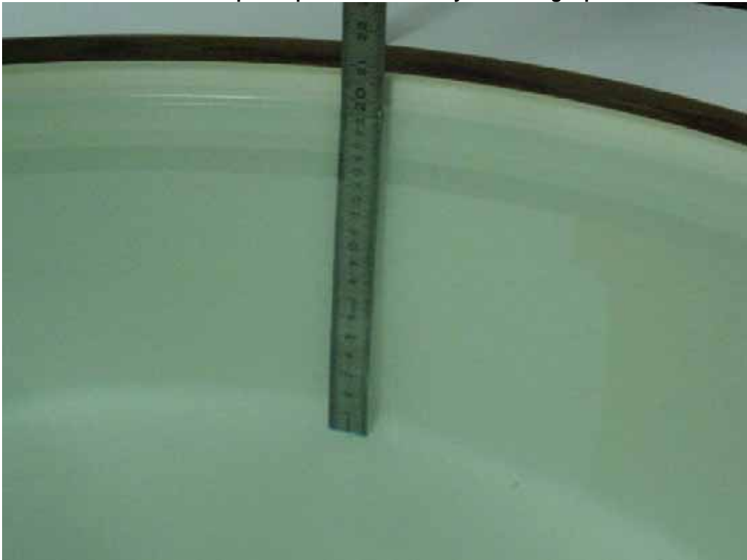
Photo 4: Liquid depth 1900 MHz body simulating liquid
