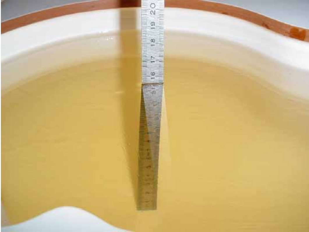
Photo 2: Liquid depth 850 MHz body simulating liquid
