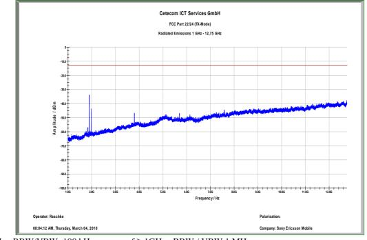
f < 1 GHz : RBW/VBW: 100 kHz Carrier suppressed with a rejection filter
