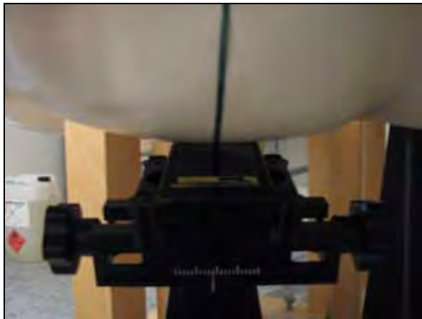
DUT position towards the head: Tilt (touch +15 deg.) position
