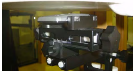
DUT position towards the body and 15 mm distance
