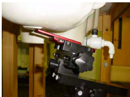
DUT position towards the head: Tilt (touch + 15°) position, Slider Open
