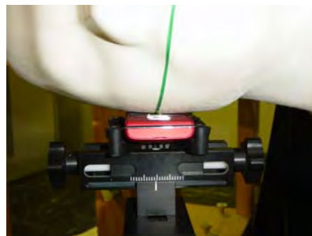
DUT position towards the head: Cheek (touch) position, Slider Closed
