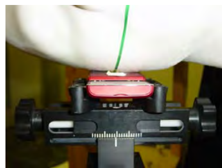
DUT position towards the head: Cheek (touch) position, Slider Open
