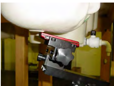
DUT position towards the head: Tilt (touch + 15°) position, Slider Closed
