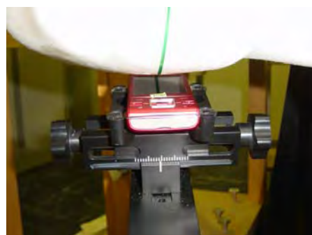
DUT position towards the head: Tilt (touch + 15°) position, Slider Closed
