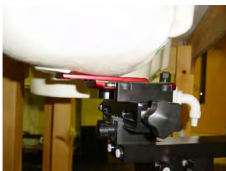
DUT position towards the head: Cheek (touch) position, Slider Open
