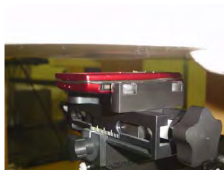
DUT position towards the body, rear and front, and 15 mm distance
