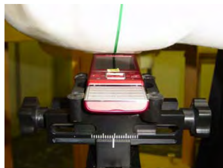
DUT position towards the head: Tilt (touch + 15°) position, Slider Open
