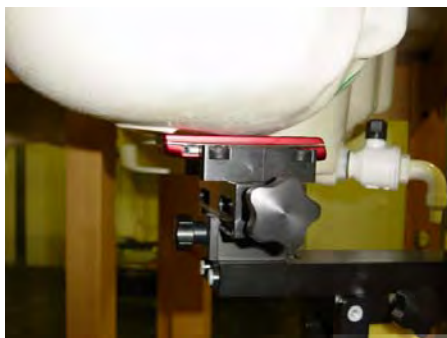
DUT position towards the head: Cheek (touch) position, Slider Closed
