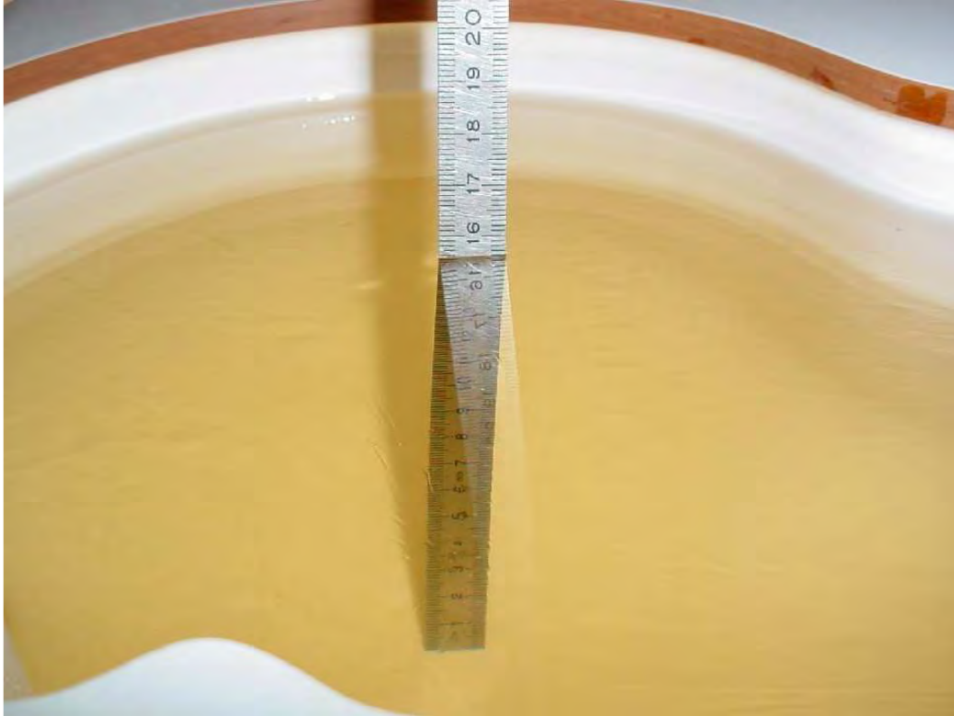
Photo 22: Liquid depth 850 MHz body simulating liquid
