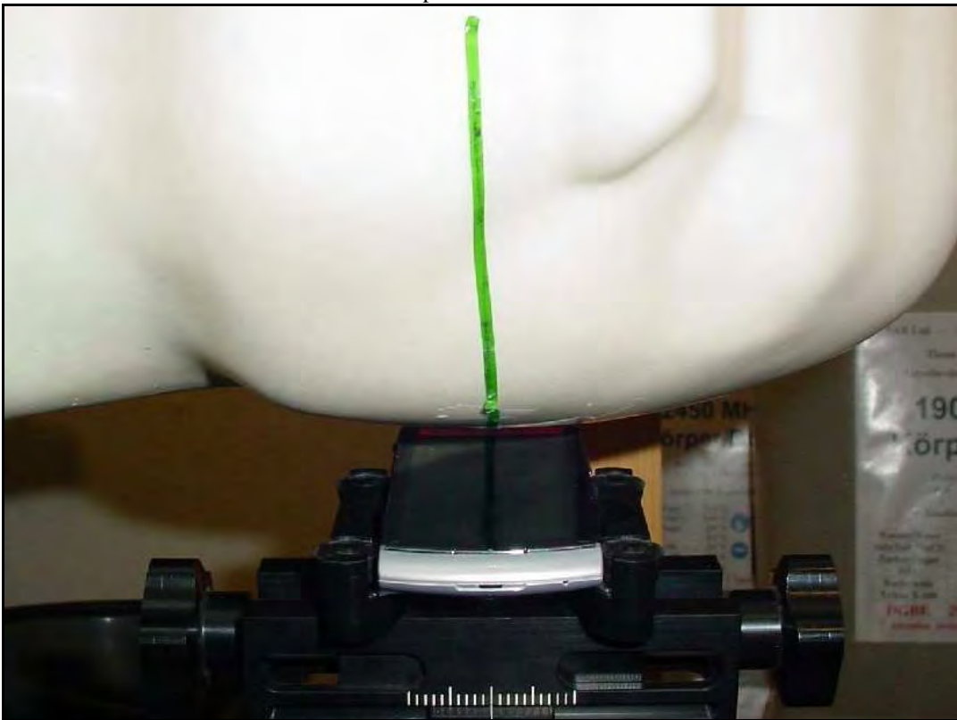
Photo 12: Test position left hand tilted 15°
