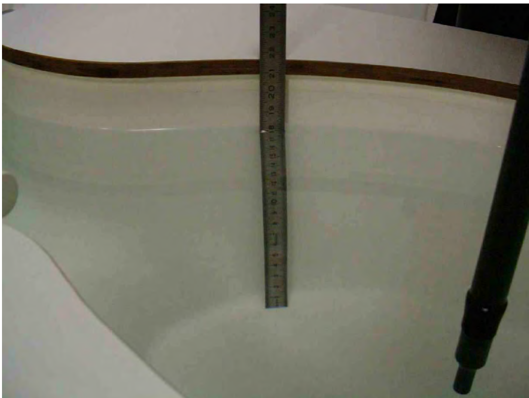
Photo 26: Liquid depth 2450 MHz body simulating liquid
