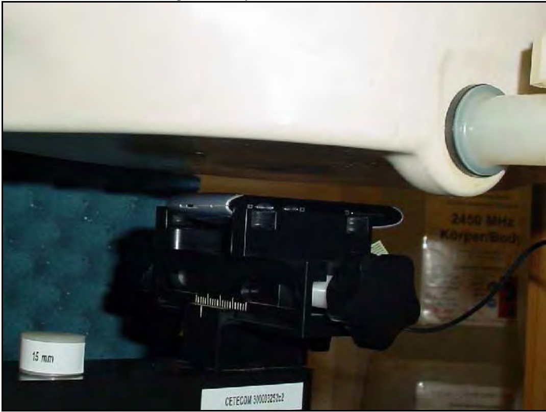
Photo 20: Test position body worn rear side with 15 mm distance
