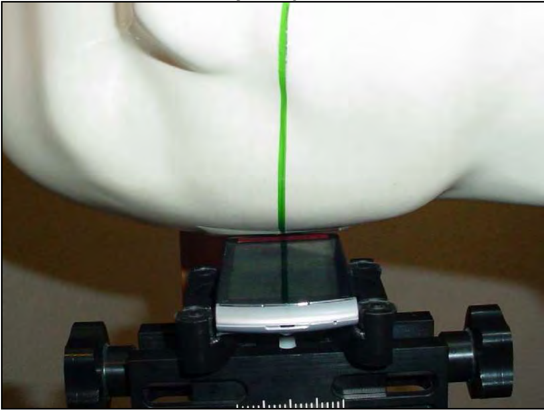
Photo 18: Test position right hand tilted 15°
