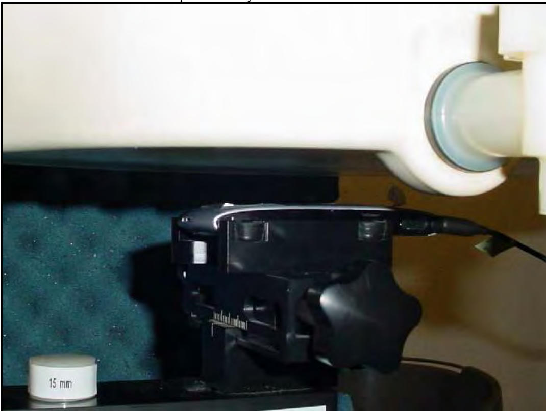
Photo 20: Test position body worn rear side with 15 mm distance
