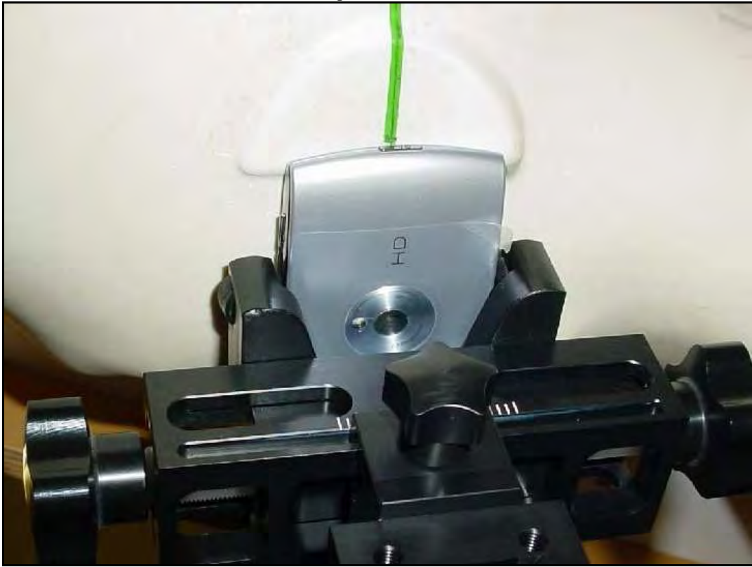
Photo 12: Test position left hand tilted 15°
