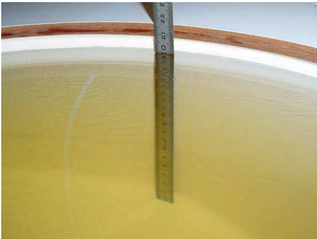
Photo 22: Liquid depth 850 MHz body simulating liquid
