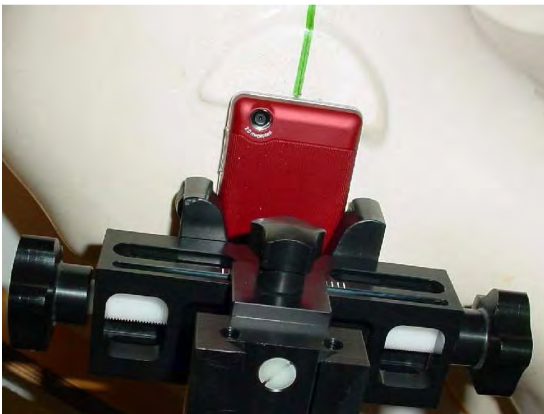
Photo 12: Test position left hand tilted 15°
