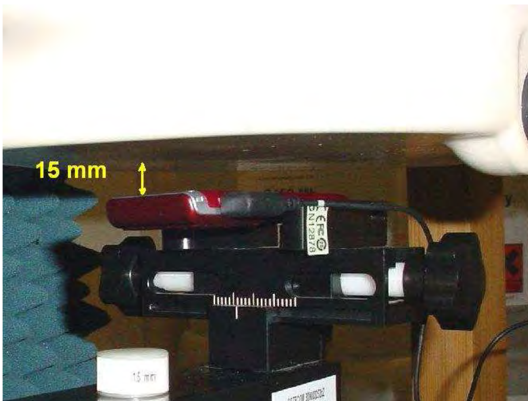
Photo 22: Test position body worn rear side (15 mm distance)
