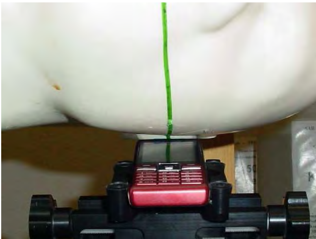
Photo 12: Test position left hand tilted 15°
