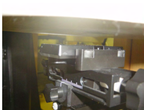
DUT position towards the body and 15 mm distance
