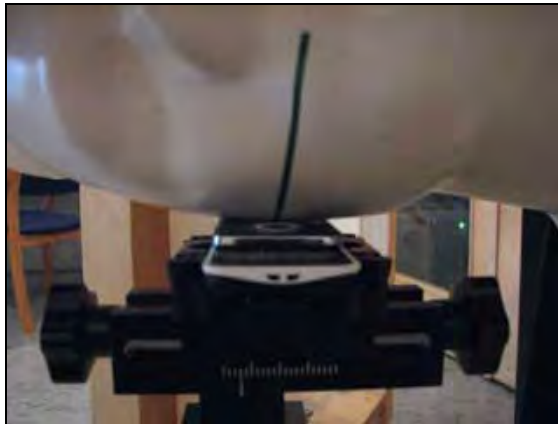
DUT position towards the head: Cheek (touch) open position
