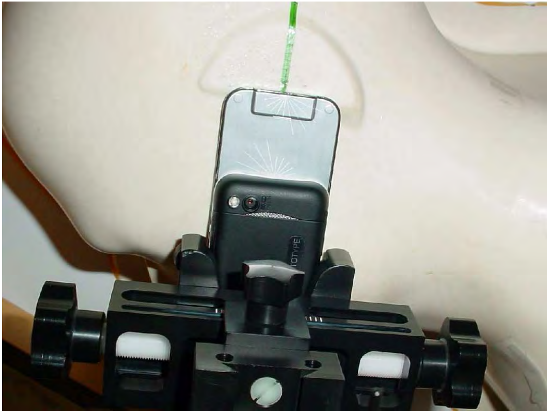
Photo 20: Test position left hand tilted 15° slide opened
