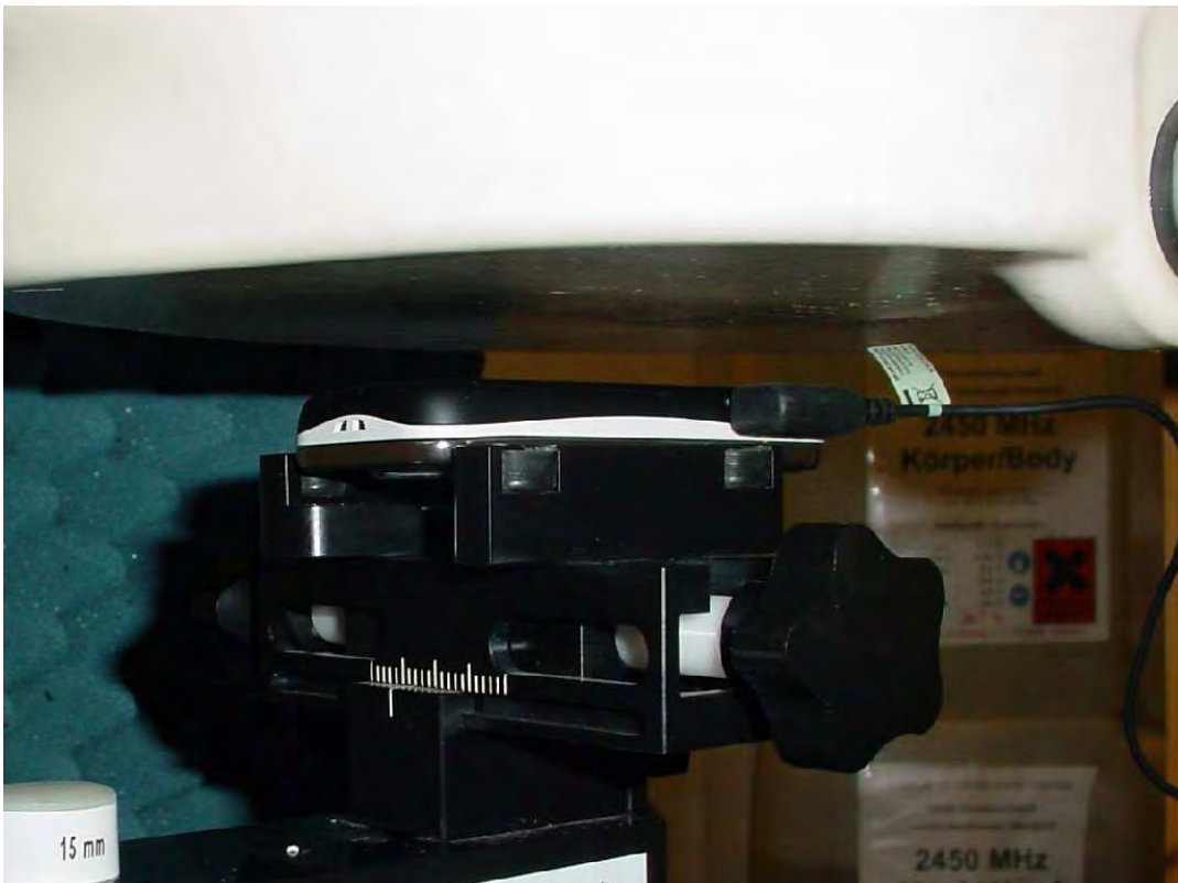
Photo 34: Test position body worn rear side with 15 mm distance
