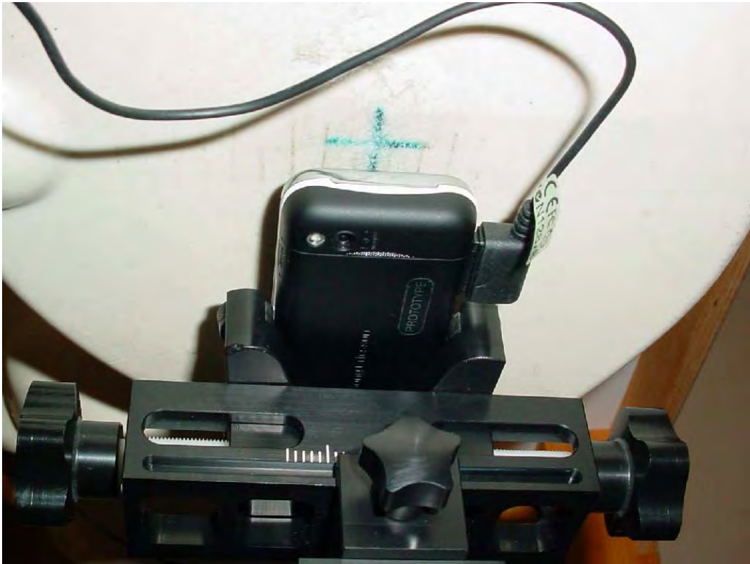
Photo 34: Test position body worn rear side with 15 mm distance
