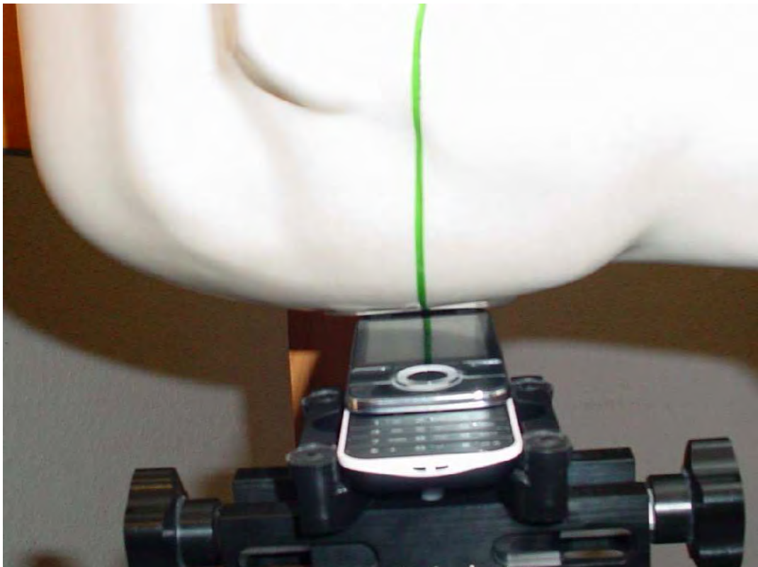
Photo 30: Test position right hand tilted 15° slide opened
