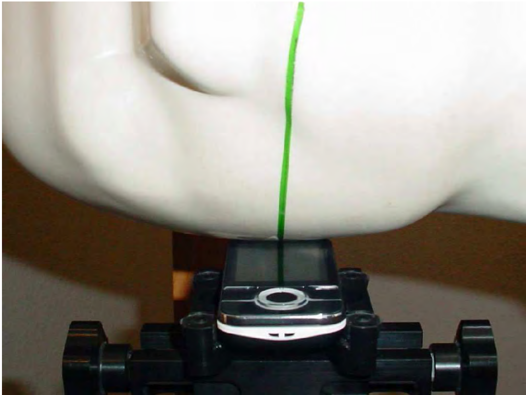
Photo 26: Test position right hand tilted 15°
