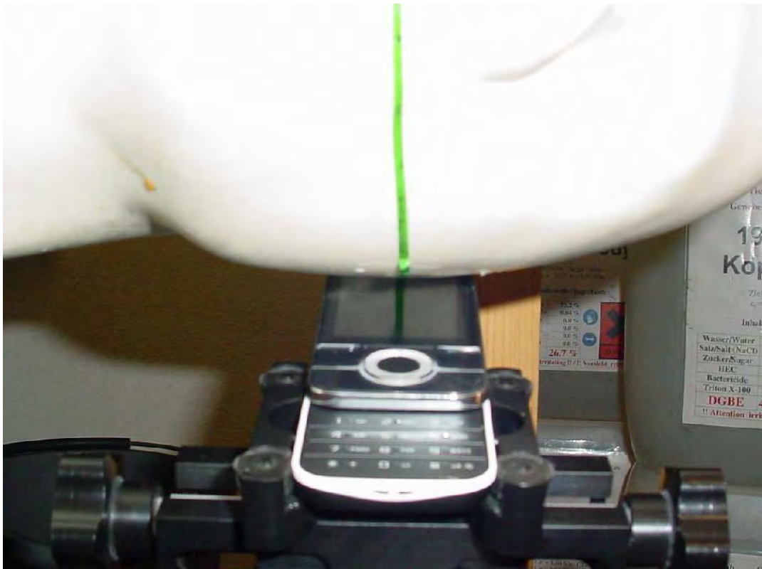
Photo 20: Test position left hand tilted 15° slide opened
