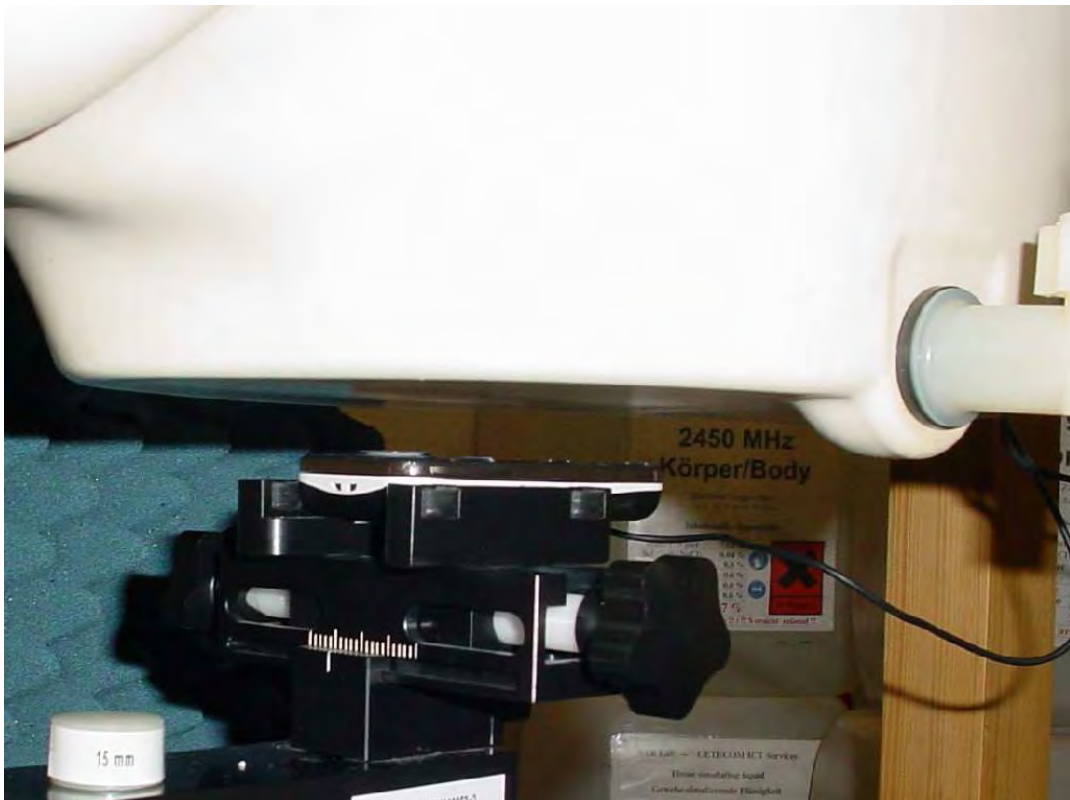
Photo 32: Test position body worn front side with 15 mm distance
