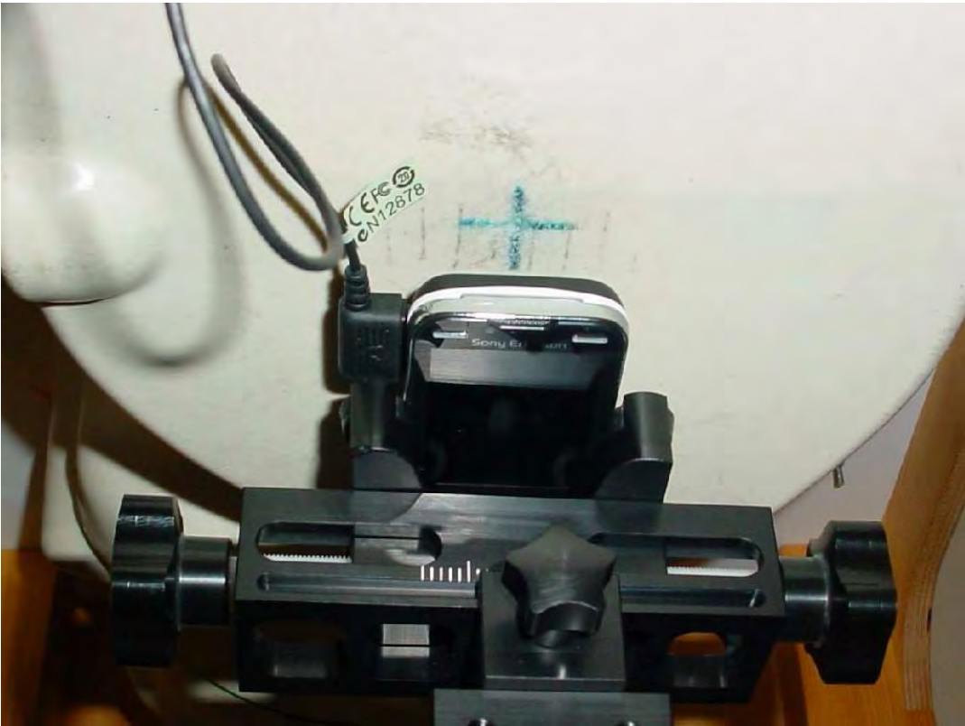
Photo 35: Test position body worn rear side with 15 mm distance
