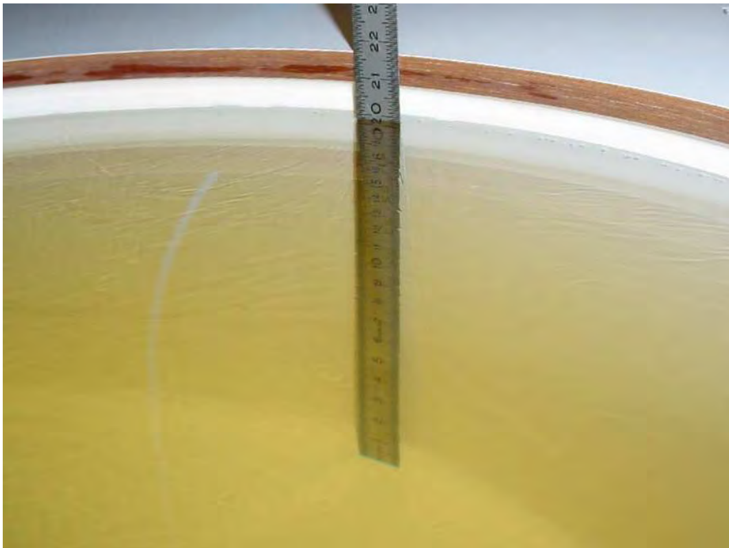
Photo 37: Liquid depth 850 MHz body simulating liquid
