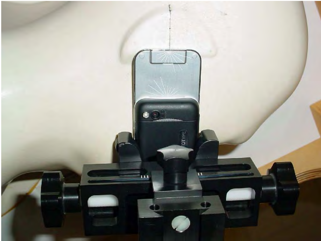
Photo 30: Test position right hand tilted 15° slide opened
