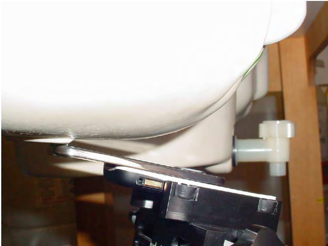
Photo 32: Test position body worn front side with 15 mm distance
