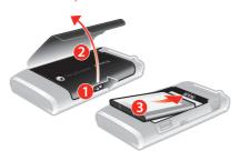
• Insert the battery with the Sony Ericsson hologram side up and the connectors facing each other.
