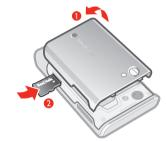
· Remove the battery cover and insert the memory card with the gold-coloured contacts facing down.
