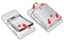
1 Insert the battery with the label side up and the connectors facing each other.
