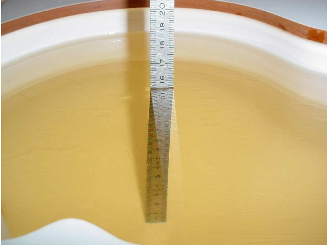
Photo 37: Liquid depth 850 MHz body simulating liquid
