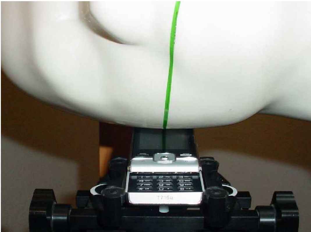
Photo 30: Test position right hand tilted 15° slide opened
