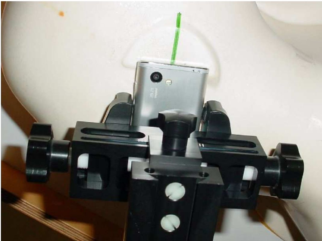
Photo 14: Test position left hand touched
