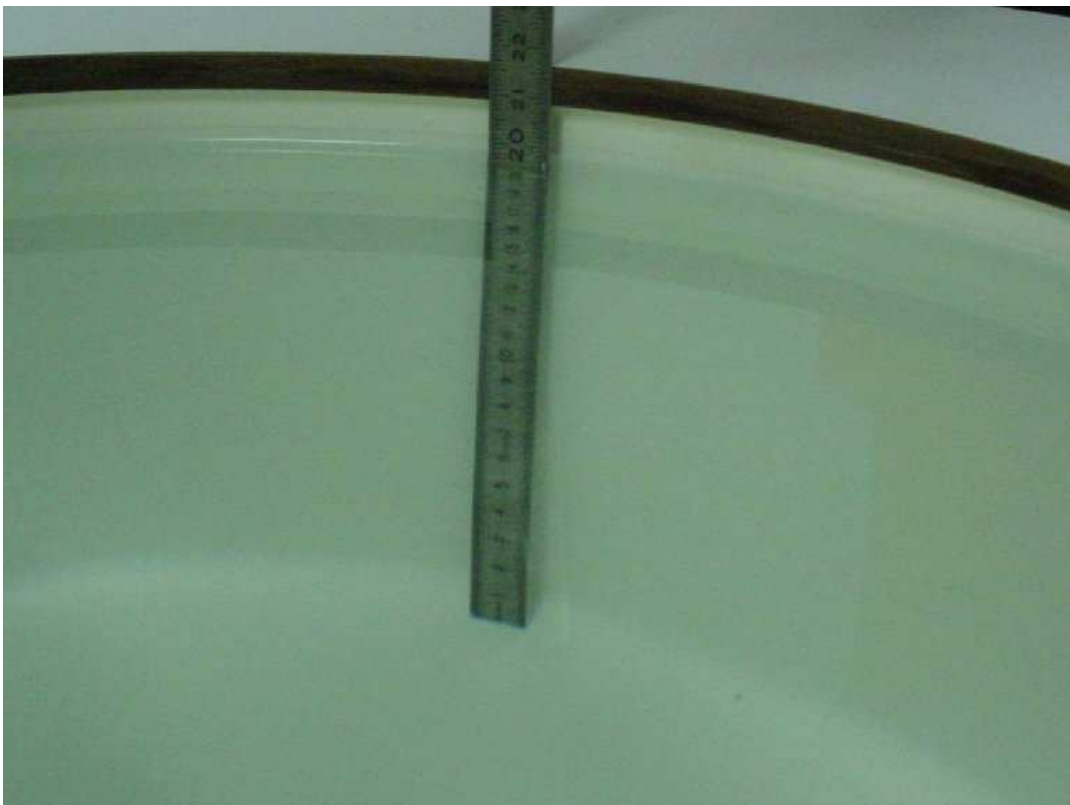
Photo 39: Liquid depth 1900 MHz body simulating liquid
