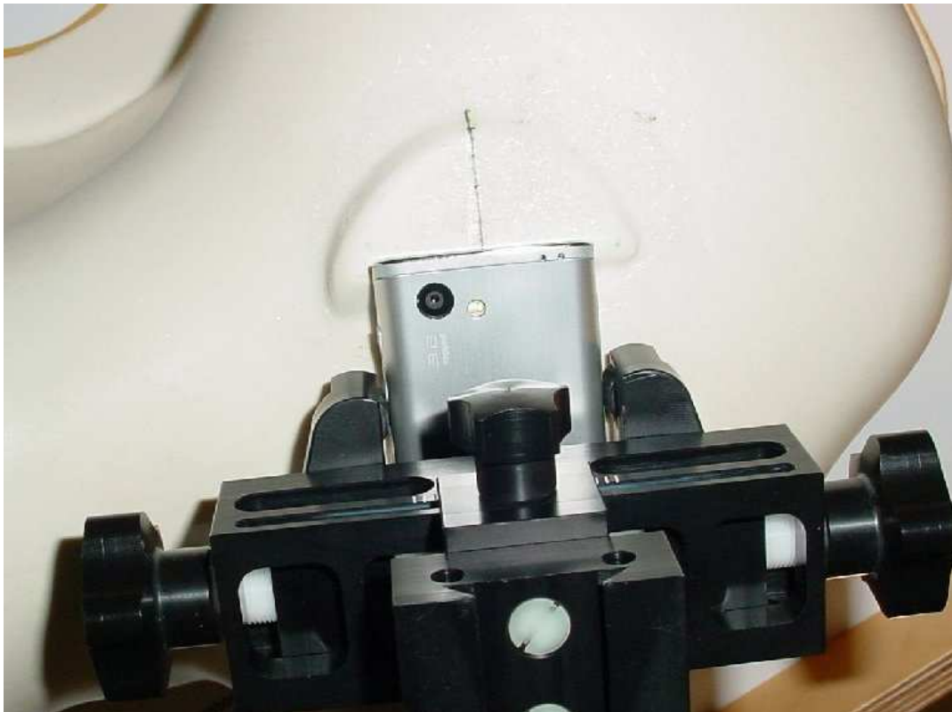
Photo 24: Test position right hand touched
