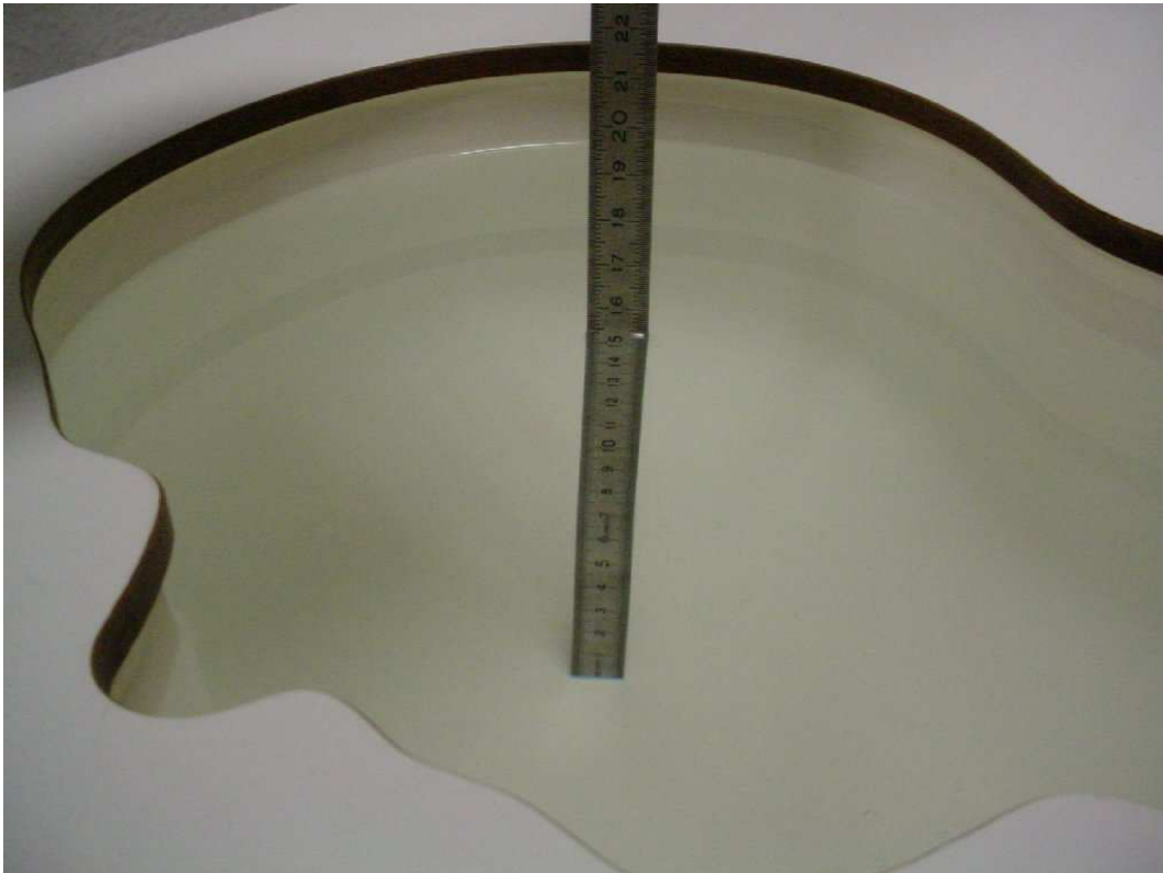
Photo 39: Liquid depth 1900 MHz body simulating liquid
