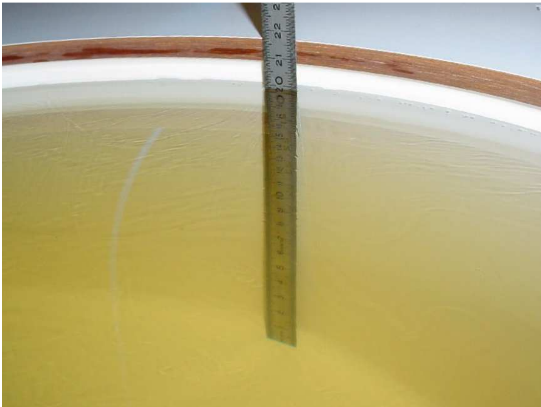
Photo 37: Liquid depth 850 MHz body simulating liquid
