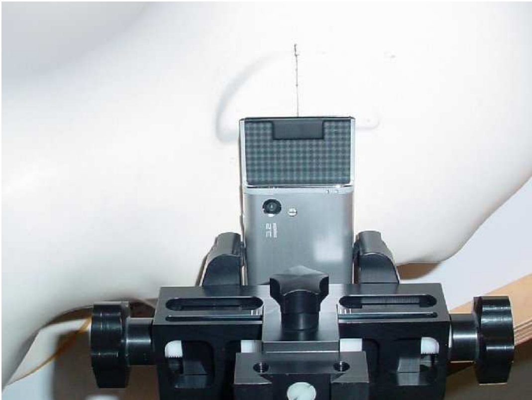
Photo 30: Test position right hand tilted 15° slide opened
