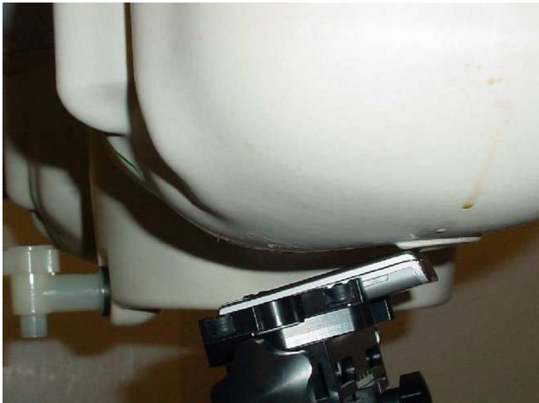
Photo 16: Test position left hand tilted 15°
